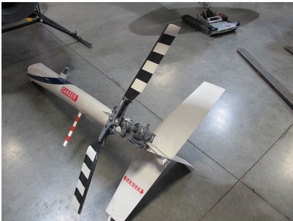
Figure 2. View of tail rotor assembly (courtesy of Robinson).
