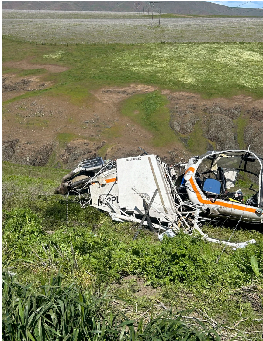
Photograph 1 - View of substantial damage to main and tail rotor systems (Courtesy of Operator)
