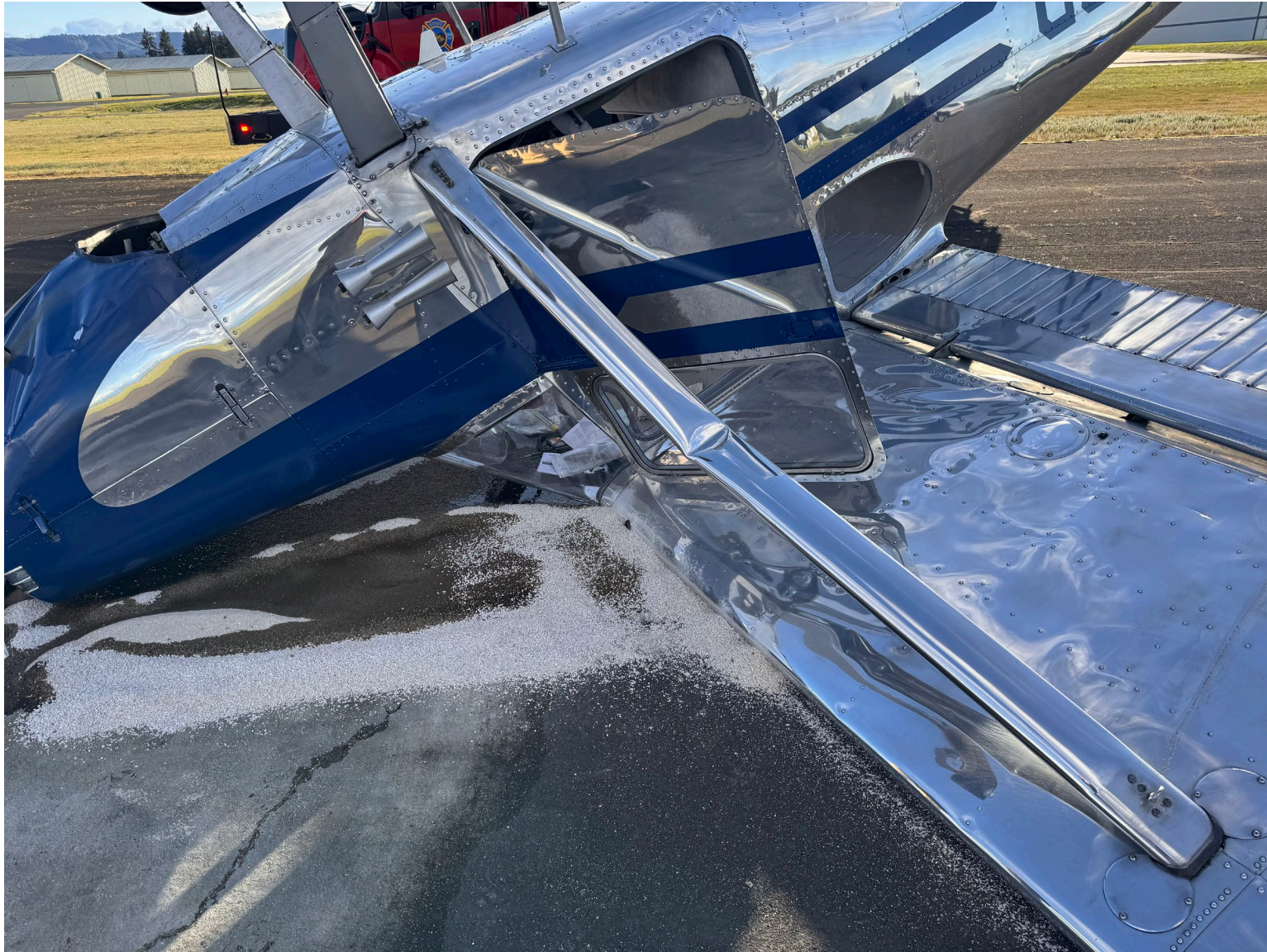
Photo 2 – View of bottom of right wing (note damage to wing strut and inboard wing) (courtesy of FAA)
