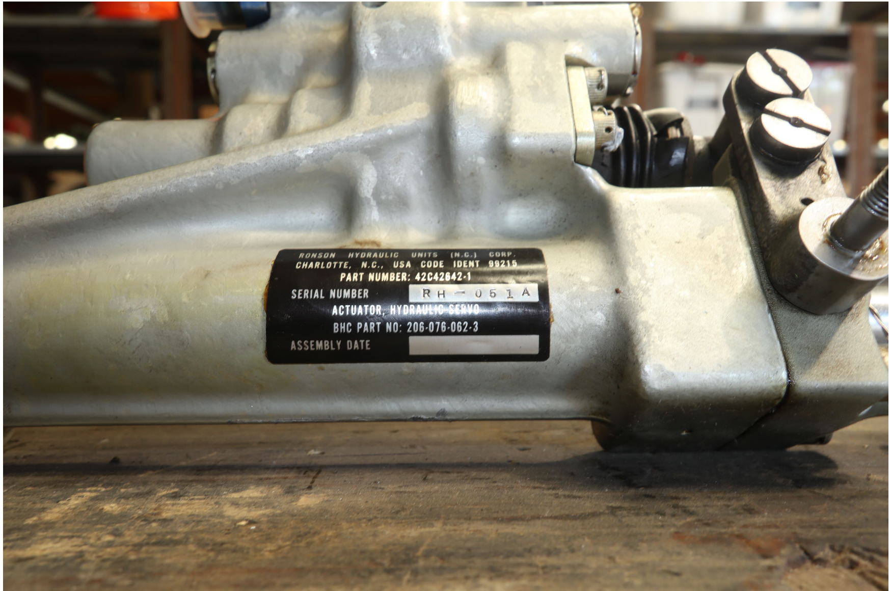
Photo 6 – Serial number of collective servo “RH-051A” (courtesy of Bell Helicopter)
