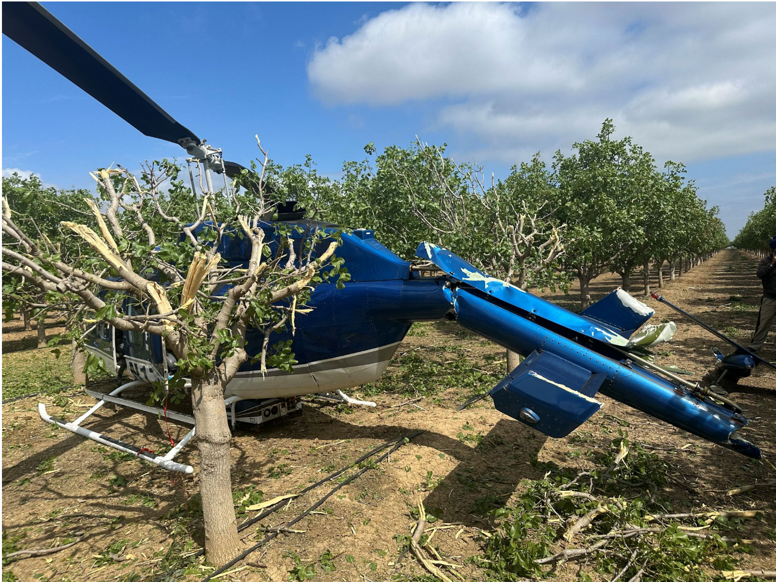
Photo 2 – View of tailboom to N17592 after accident (courtesy of Tracy Police Department)
