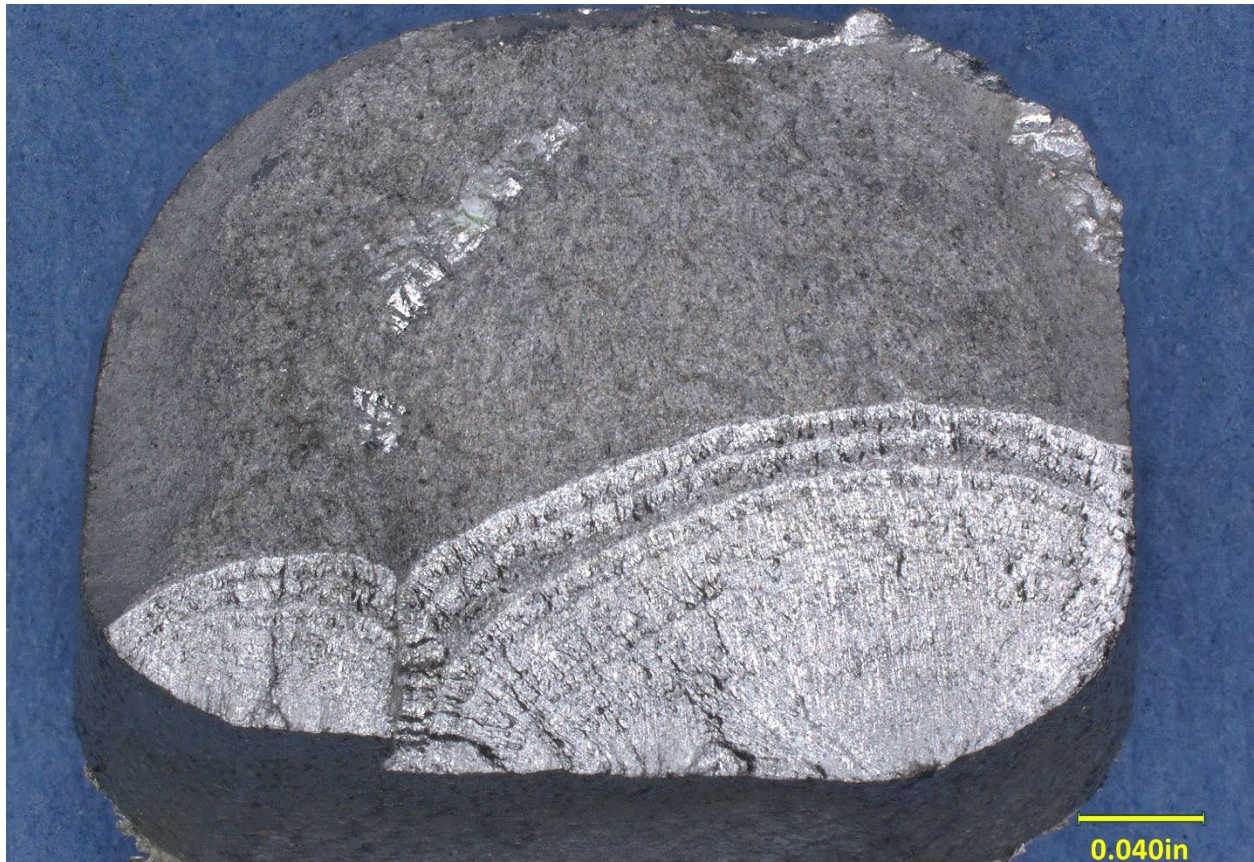
Figure 10. Upper leg fracture surface from the forward face.
