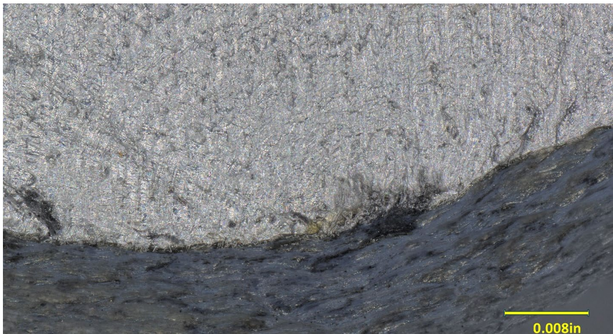
Figure 11. Primary crack initiation site of the larger crack in Figure 10.
