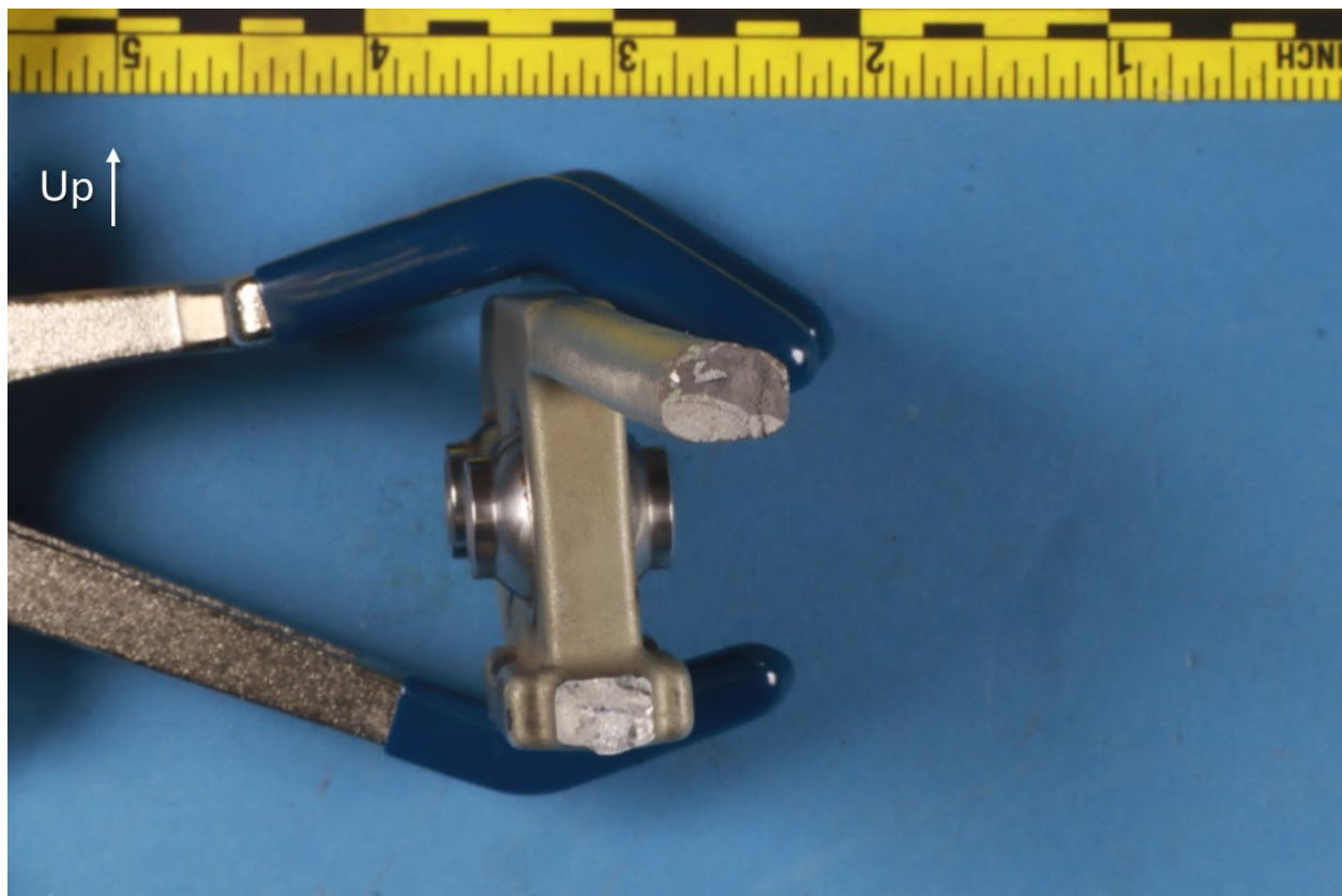
Figure 5. View of the two fracture surfaces of the servo arm, from the forward-looking aft view.
