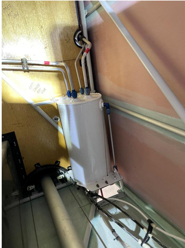
Photograph 8 - Header Fuel Tank, Mid-Fuselage (NTSB photo)
