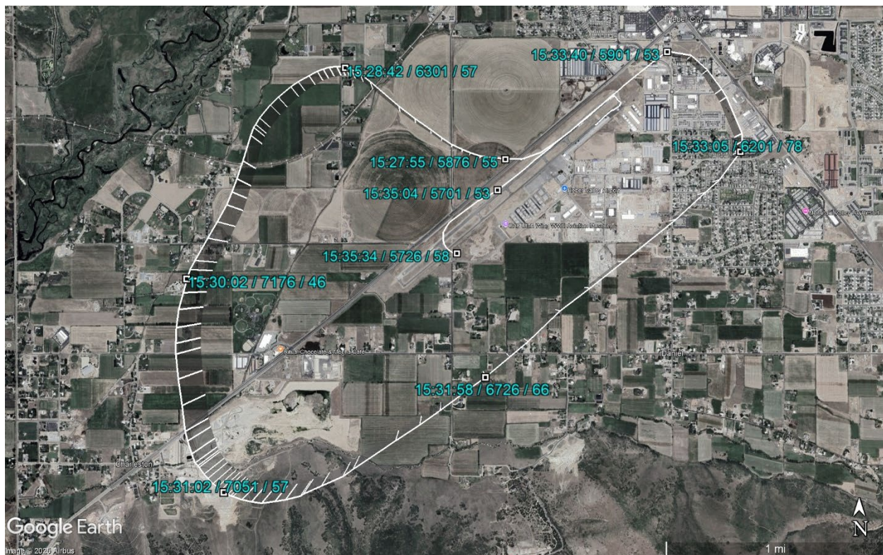
Figure 2. Overhead view of the entire flight on a Google Earth background. Annotations indicate time MDT, MSL altitude and groundspeed. Both takeoffs were to the southwest on runway 22.
