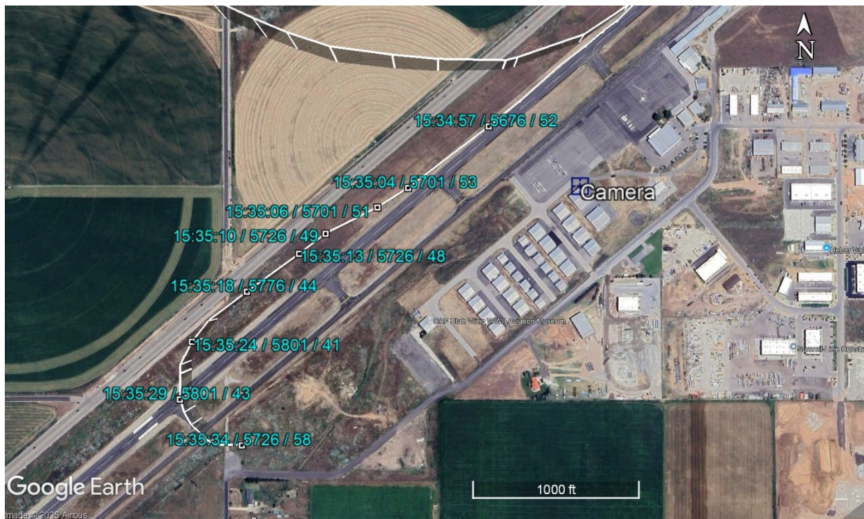
Figure 2. Accident flight track from ADS-B data on a Google Earth background. The position of the camera on an airport building is indicated. Annotations on the flight track show the time MDT, altitude above mean sea level in feet and groundspeed in knots.
