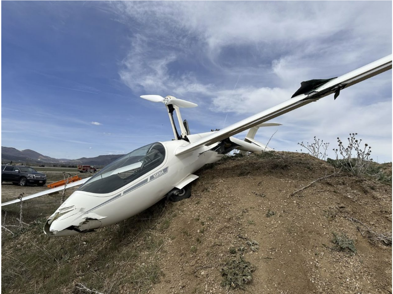
Figure 2. Substantial fuselage and wing damage. Photo courtesy of the pilot.
