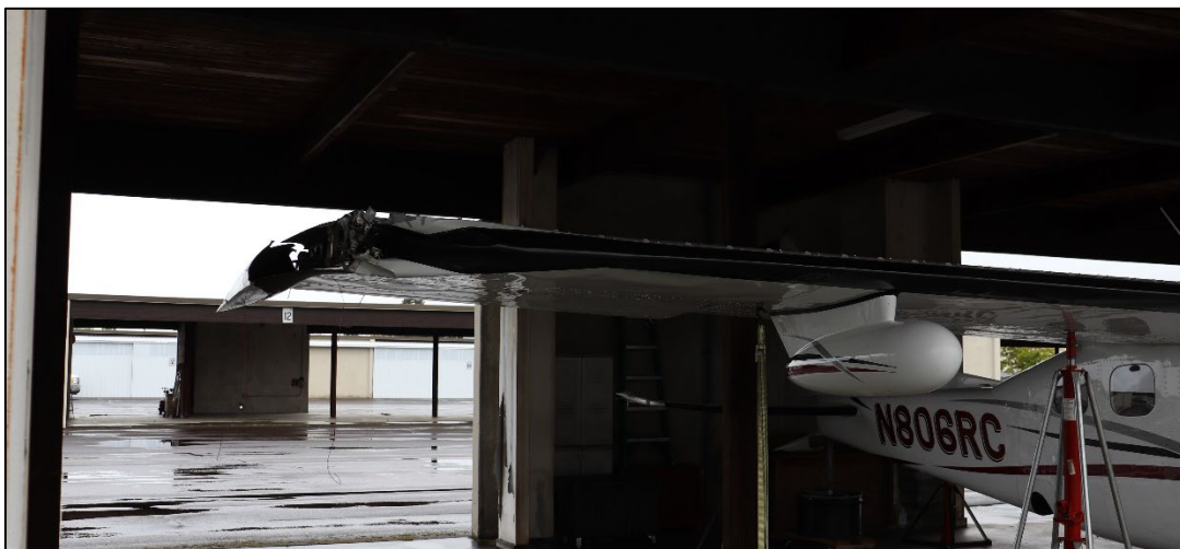
Figure 2: View of right wing tip damage.
