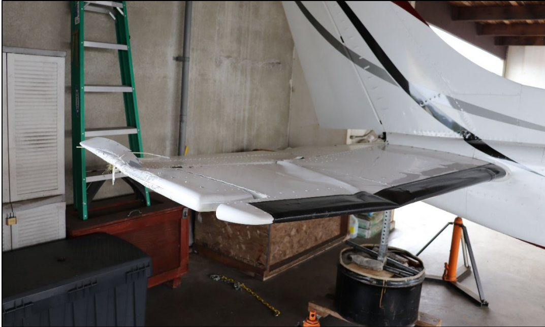
Figure 3: View of right horizontal stabilizer and elevator damage.
