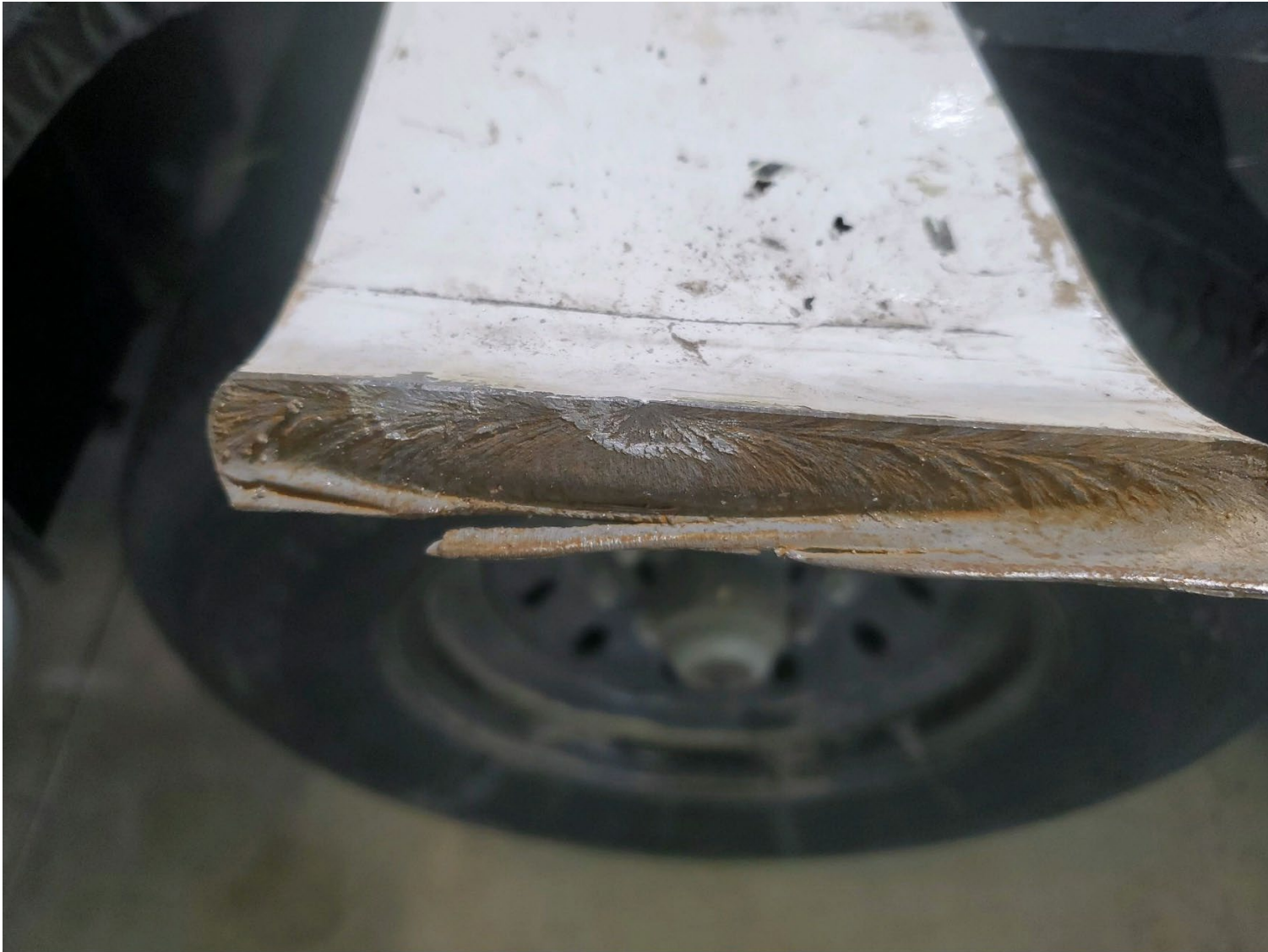
Photograph 4 - View of gear spring inboard fracture (wheel-side)
