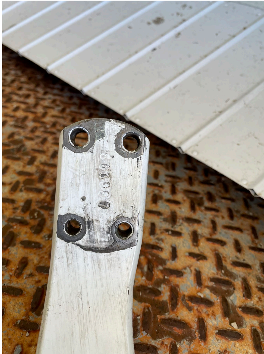
Photograph 3 - View of outboard gear spring
