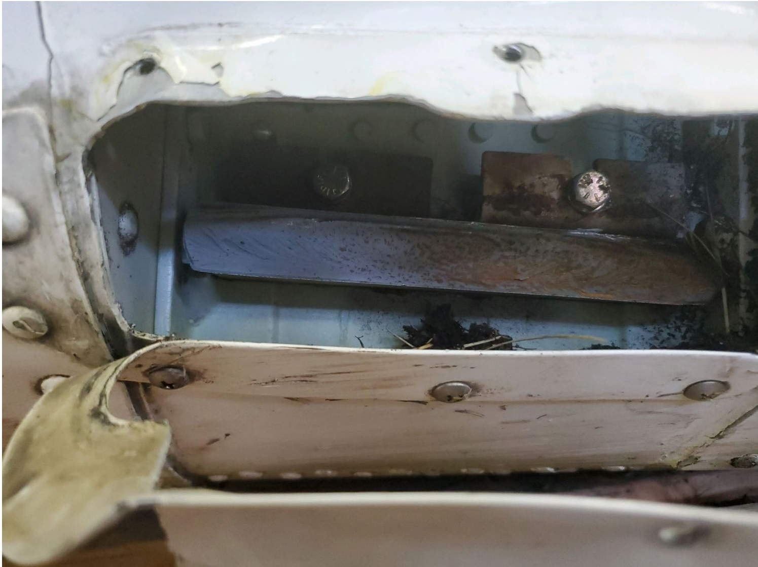
Photograph 5 - View of gear spring inboard fracture (planeside)
