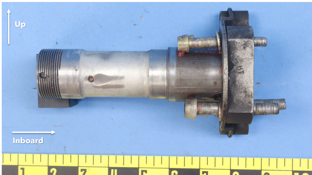
Figure 4. Aft-looking forward view of the axle assembly, as received.
