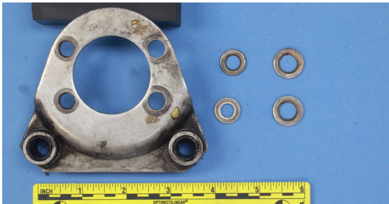
Figure 11. View of the washers and faying surface of the axle, showing annular areas of fretting.
