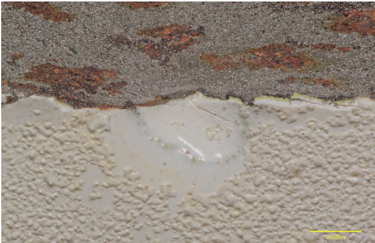
Figure 17. Angled view of the pit in Figure 16, showing paint adhering to the pit surface.
