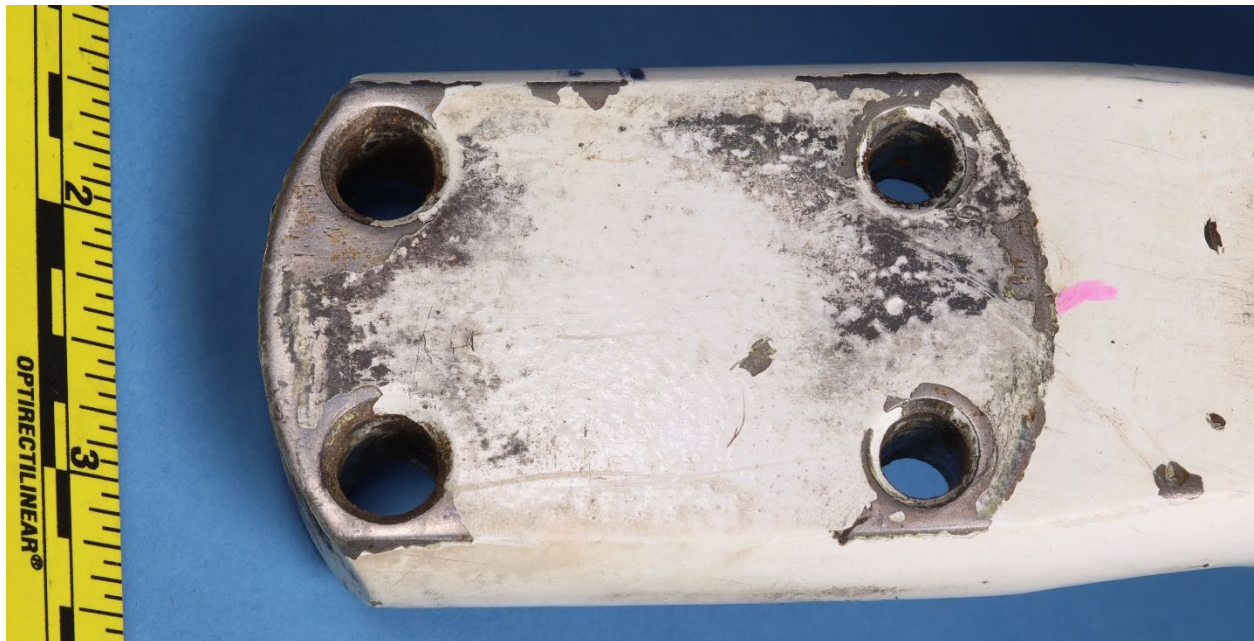
Figure 2. The outboard face of the leg from Figure 1a with the attachment bolt holes.
