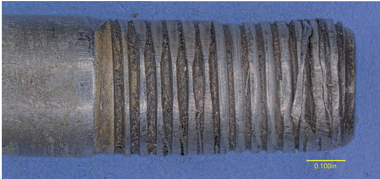
Figure 12. Side view of the damaged threads from the aft lower bolt.
