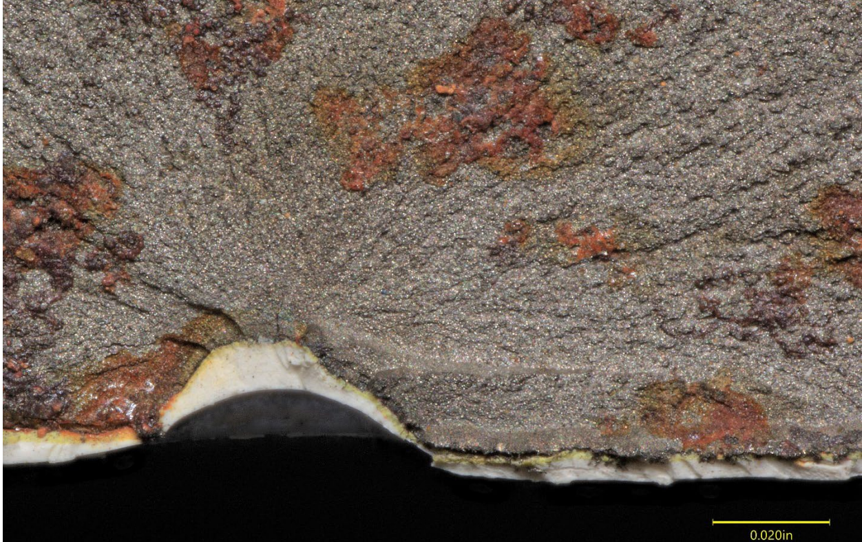
Figure 16. Closer view of the pit and fatigue cracking at the initiation of the leg fracture.
