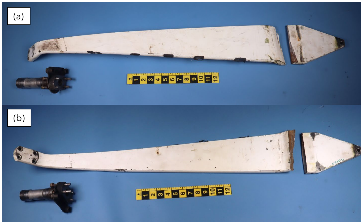
Figure 1. The pieces of the left landing gear leg, as received from (a) outboard and (b) inboard faces.
