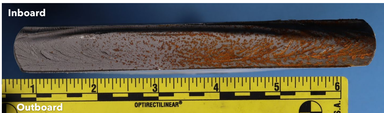
Figure 14. View of the outboard fracture surface of the landing gear leg, as received.
