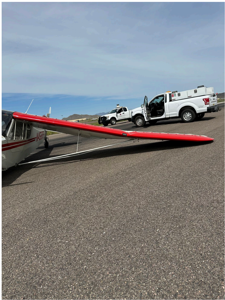
Photo 1 – View of left wing damage (Photo courtesy of pilot)
