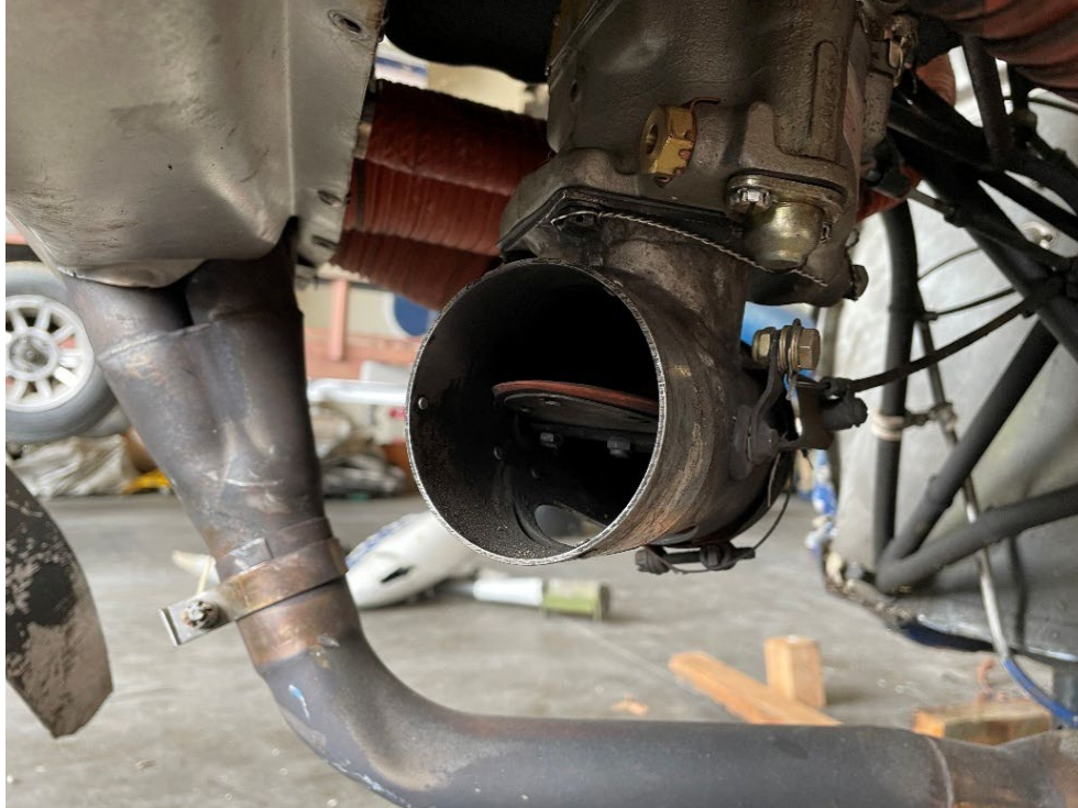
Fig. 5: View of cable attachment at airbox and heat door with the carburetor heat at its full OFF position.
