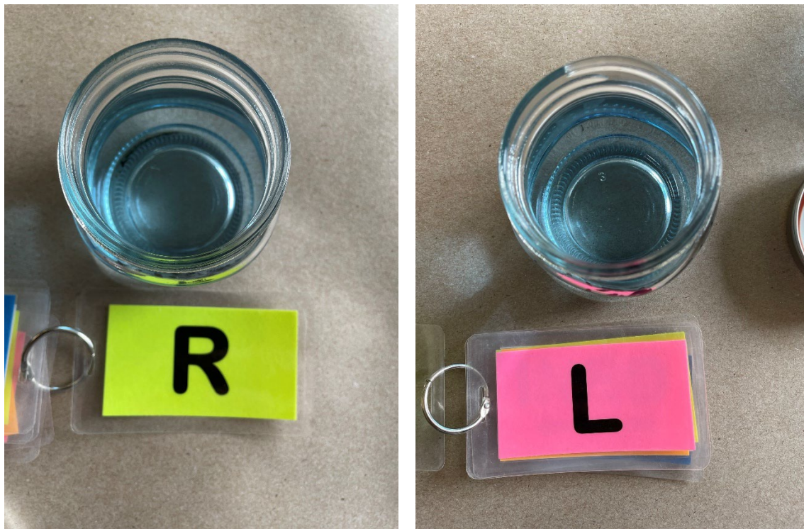
Figure 1: View of sample drained from right fuel tank. Figure 2: View of sample drained from left fuel tank.
