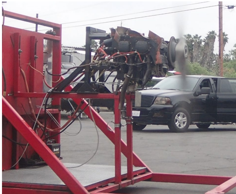
Fig. 9: View of engine on test stand during test run.
