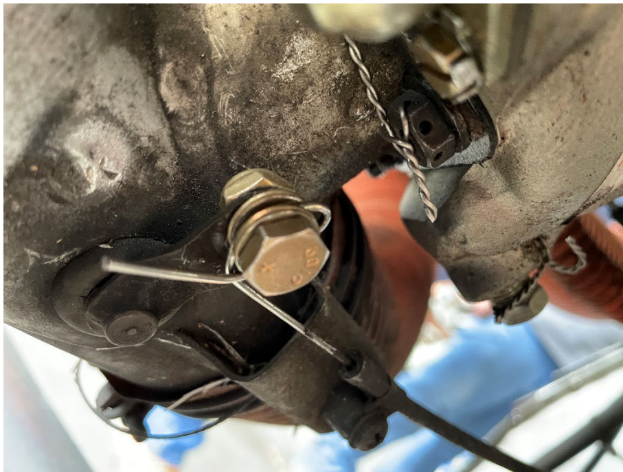
Figure 3: View of cable attachment at airbox.
