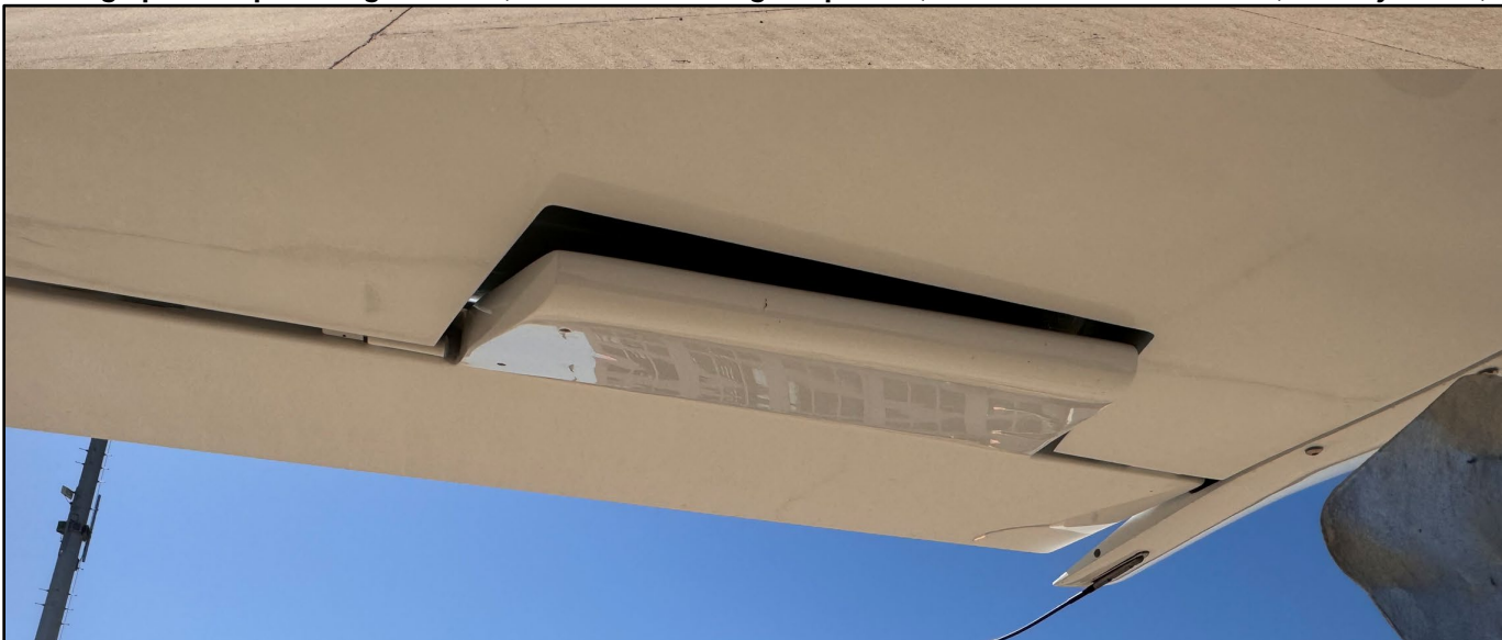
Photograph 2 - Airplane's left aileron (attached counterbalance-weight) as viewed from the bottom. (Courtesy of FAA)
