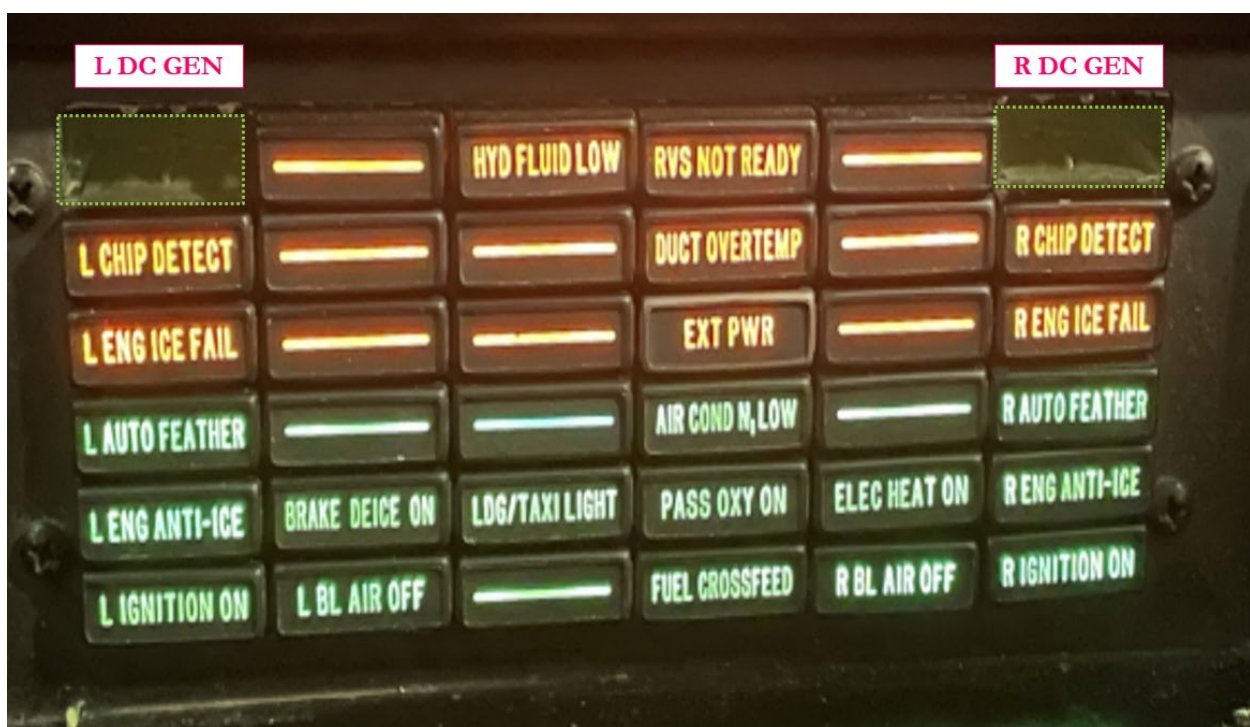
Figure 7: Test for the caution-advisory annunciation panel
