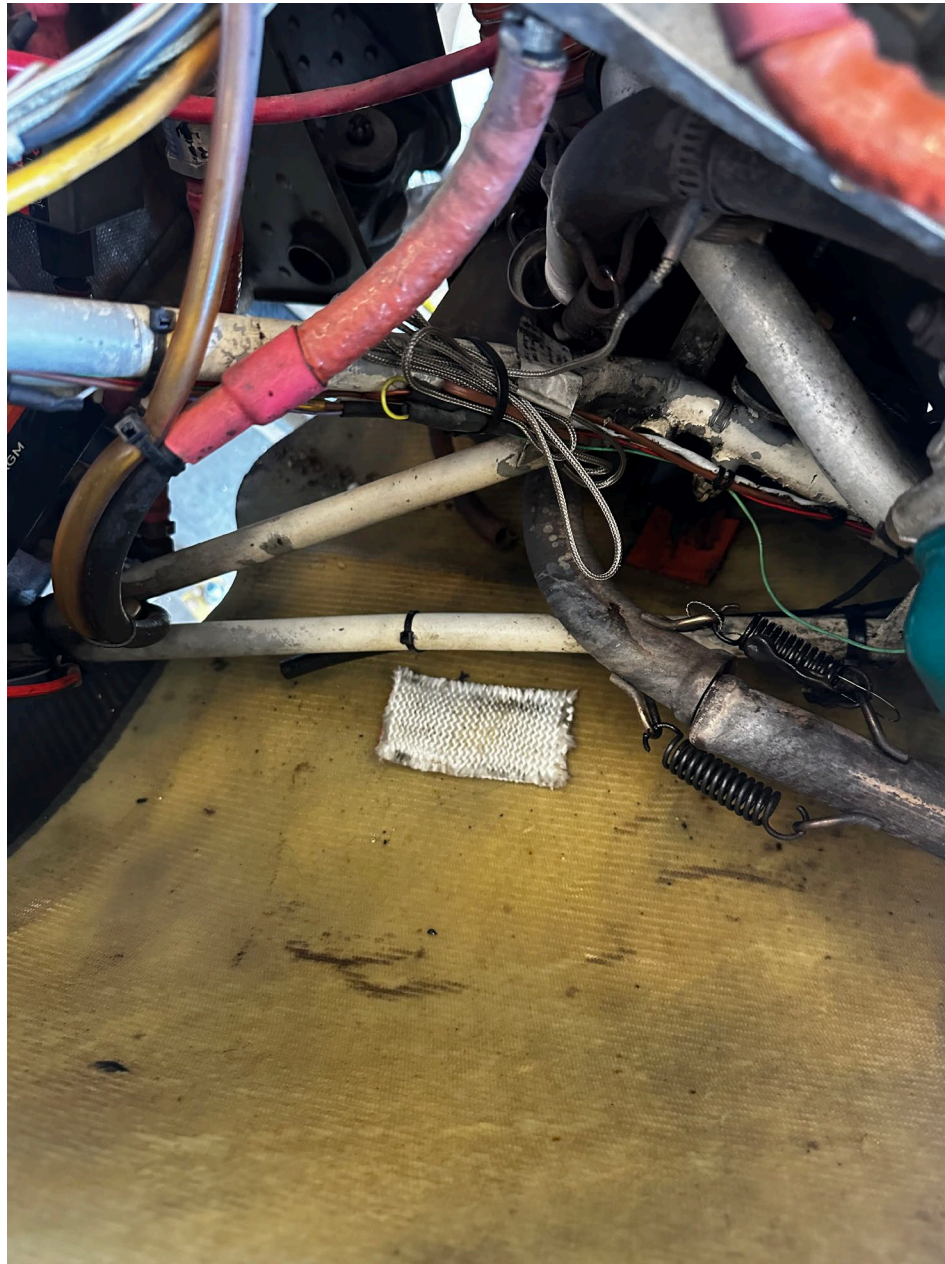
Photo 2 – Damaged engine mount. Photo courtesy of the owner.
