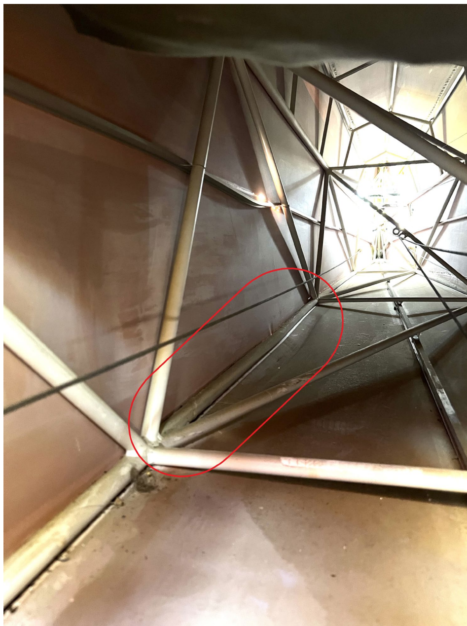
Photo 1 – View of fuselage damage (photo provided by pilot)
