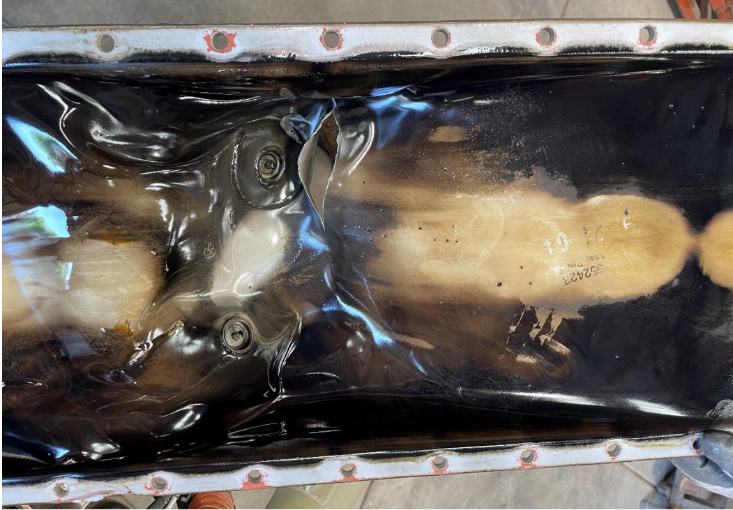
Figure 6: View of puncture in oil sump.
