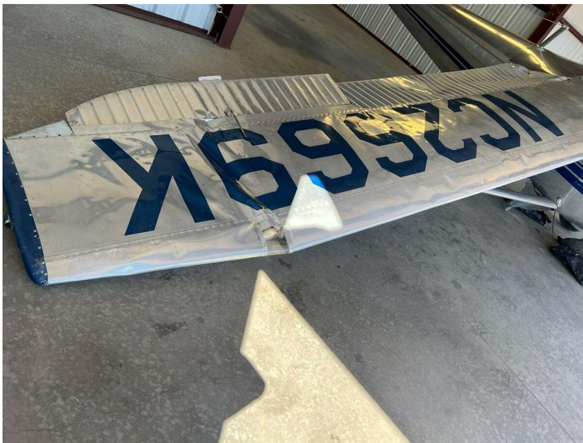
Photograph 1 - View of Damaged Wing (Courtesy of FAA)
