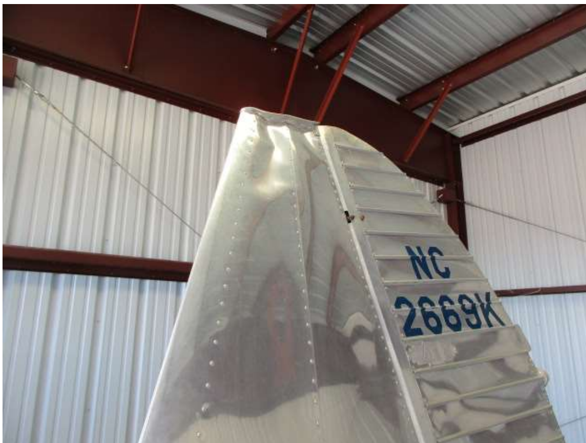
Photograph 2 - View of Damage to the Tail (Courtesy of FAA)
