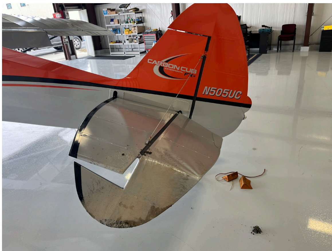
Photograph 2 - View of left elevator damage (Courtesy of the FAA)
