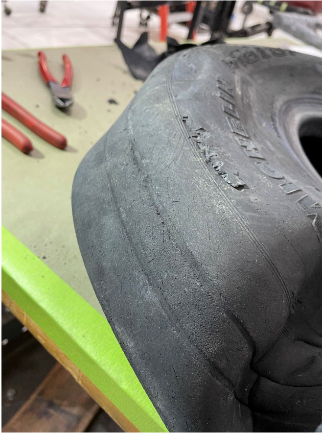
Figure 2 - Right Main Tire Tread (FAA Photo)
