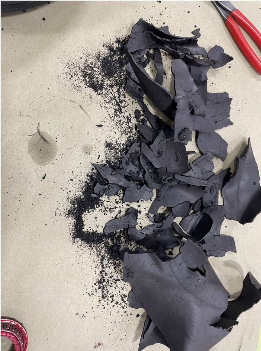
Figure 4 - Tire Inner Tube Remnants (FAA Photo)
