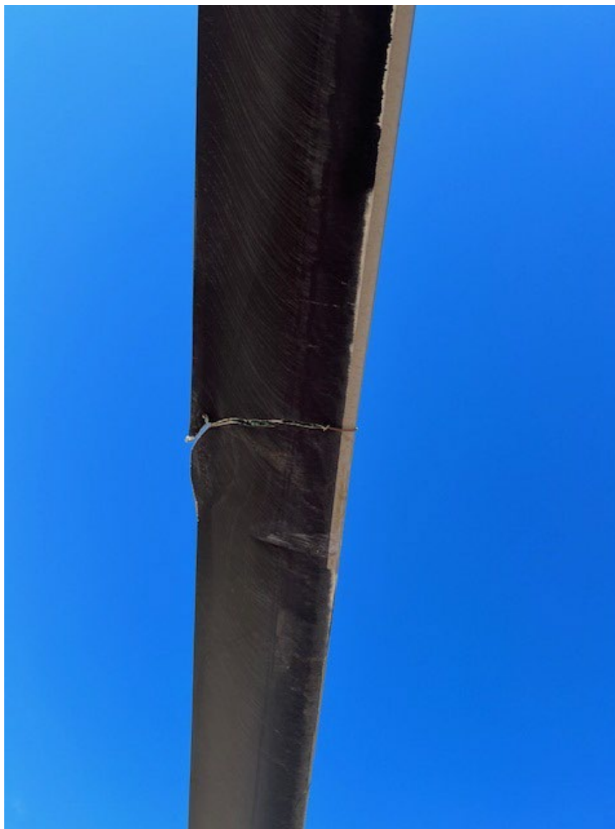
Photograph 1 - View of damage to main rotor blade (Courtesy of operator)
