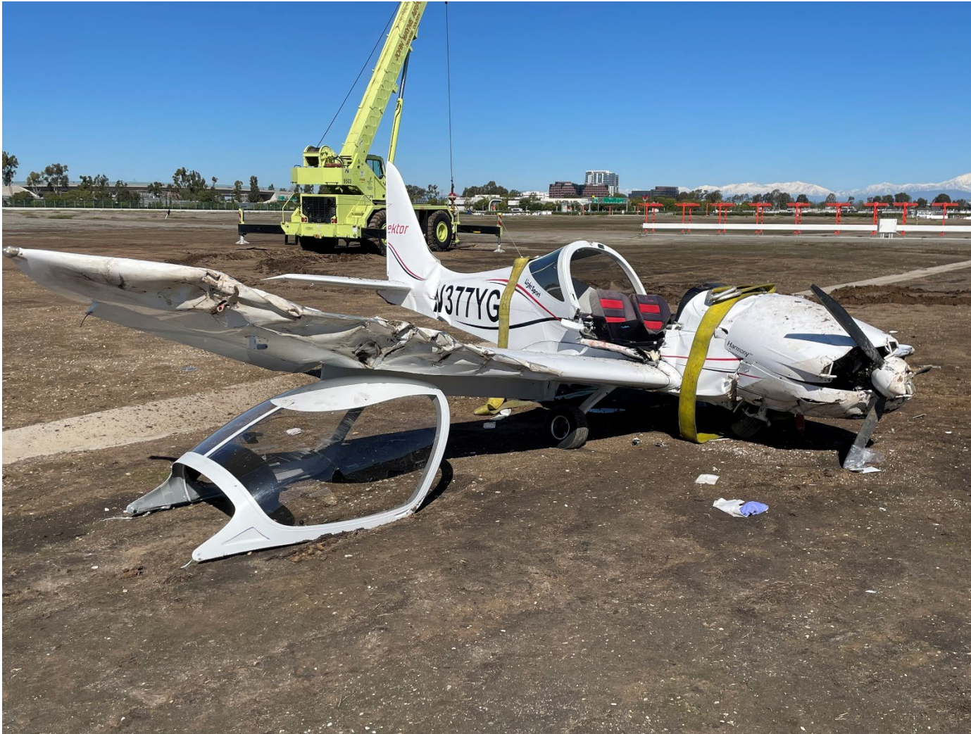
Photograph 2 - View of substantial damage to the airplane's right wing and fuselage (Courtesy of Airport Operations)
