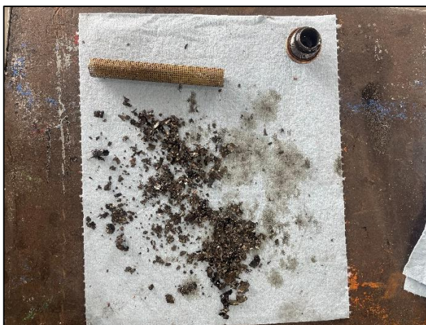
Figure 4-Oil suction screen and contaminants.
