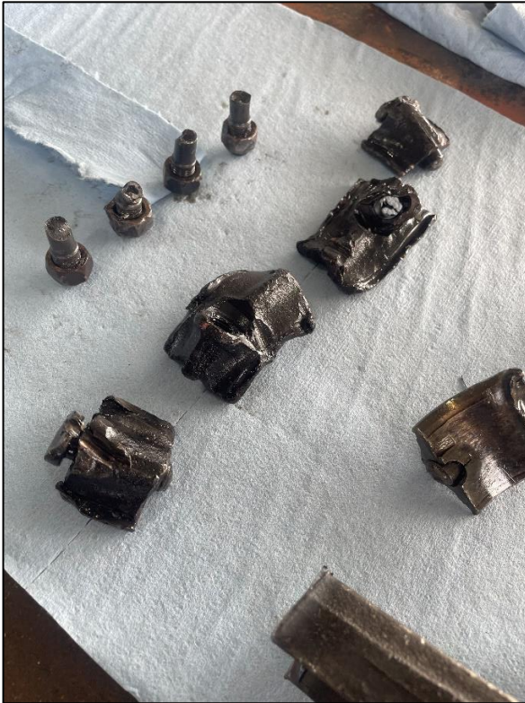
Figure 10-No. 3 connecting rod parts.
