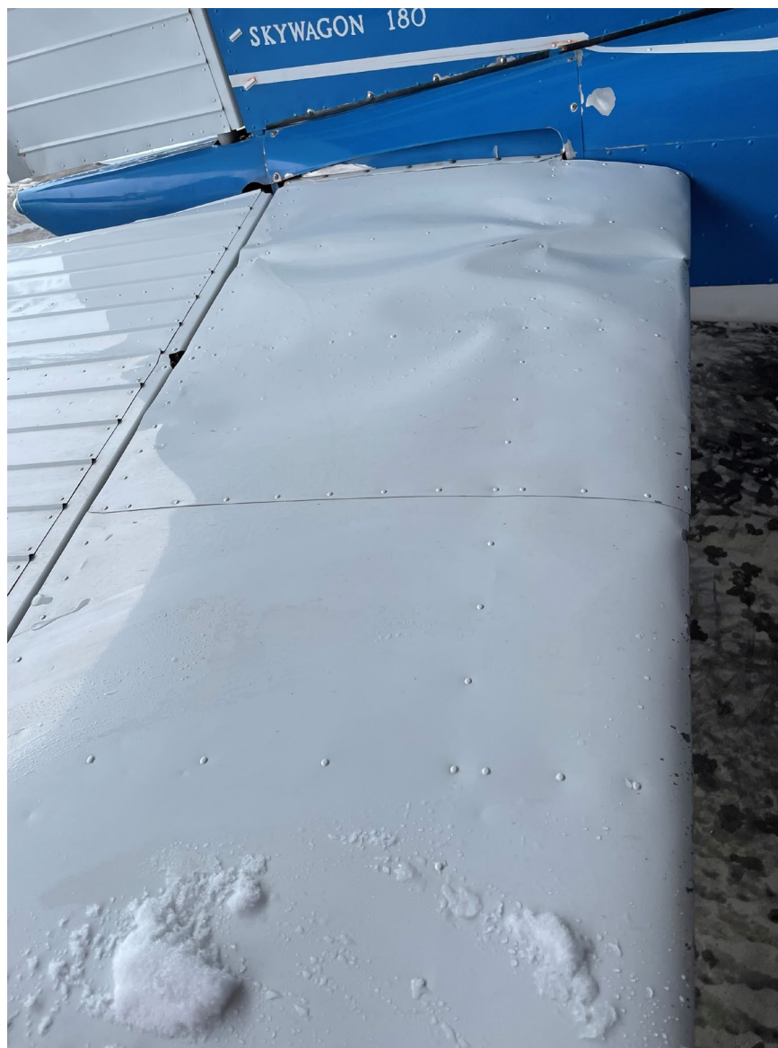
Photograph 1 - View of right horizontal stabilizer damage (Courtesy of Pilot)
