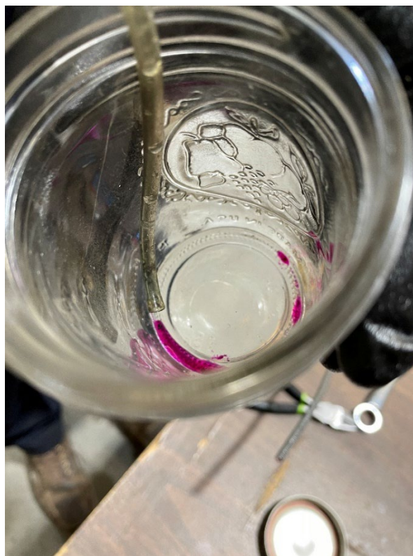
Figure 4 - Water in line (red indicates water)
