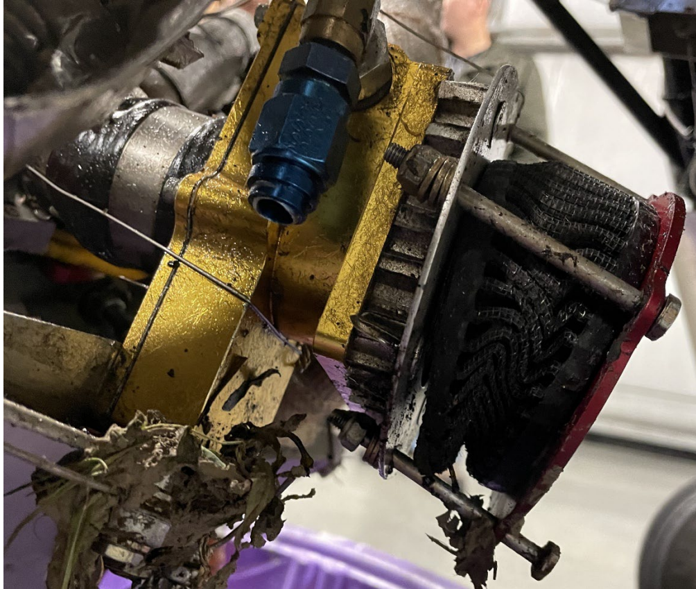
Figure 6 - Air filter and honeycomb spacer
