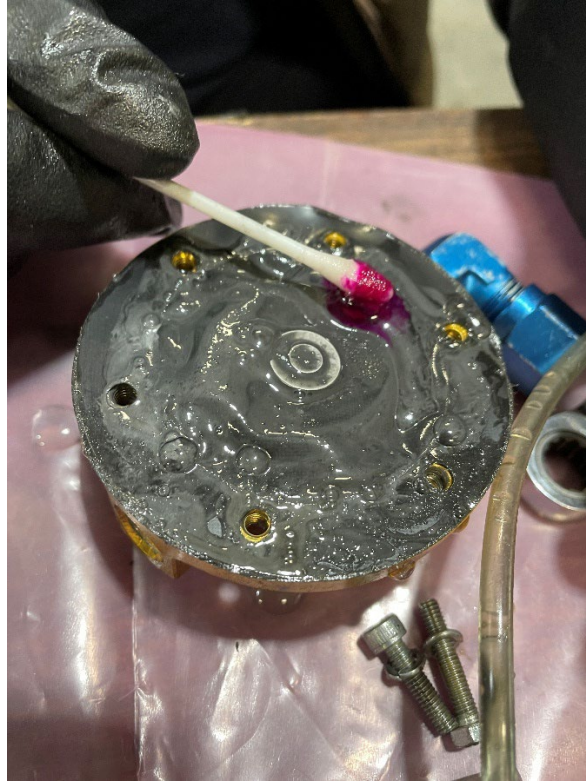
Figure 5 - Water on air side of regulator diaphragm (red indicates water)
