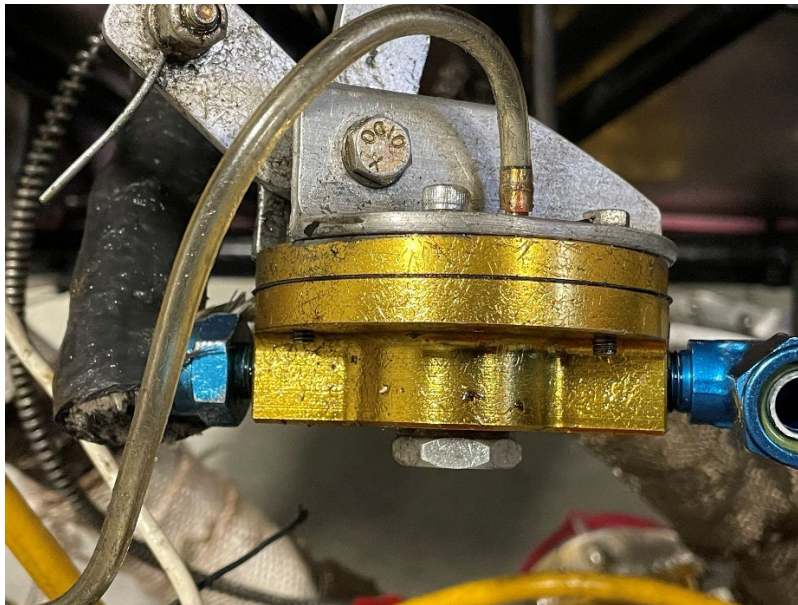
Figure 3 - Throttle body-to-regulator line containing water
