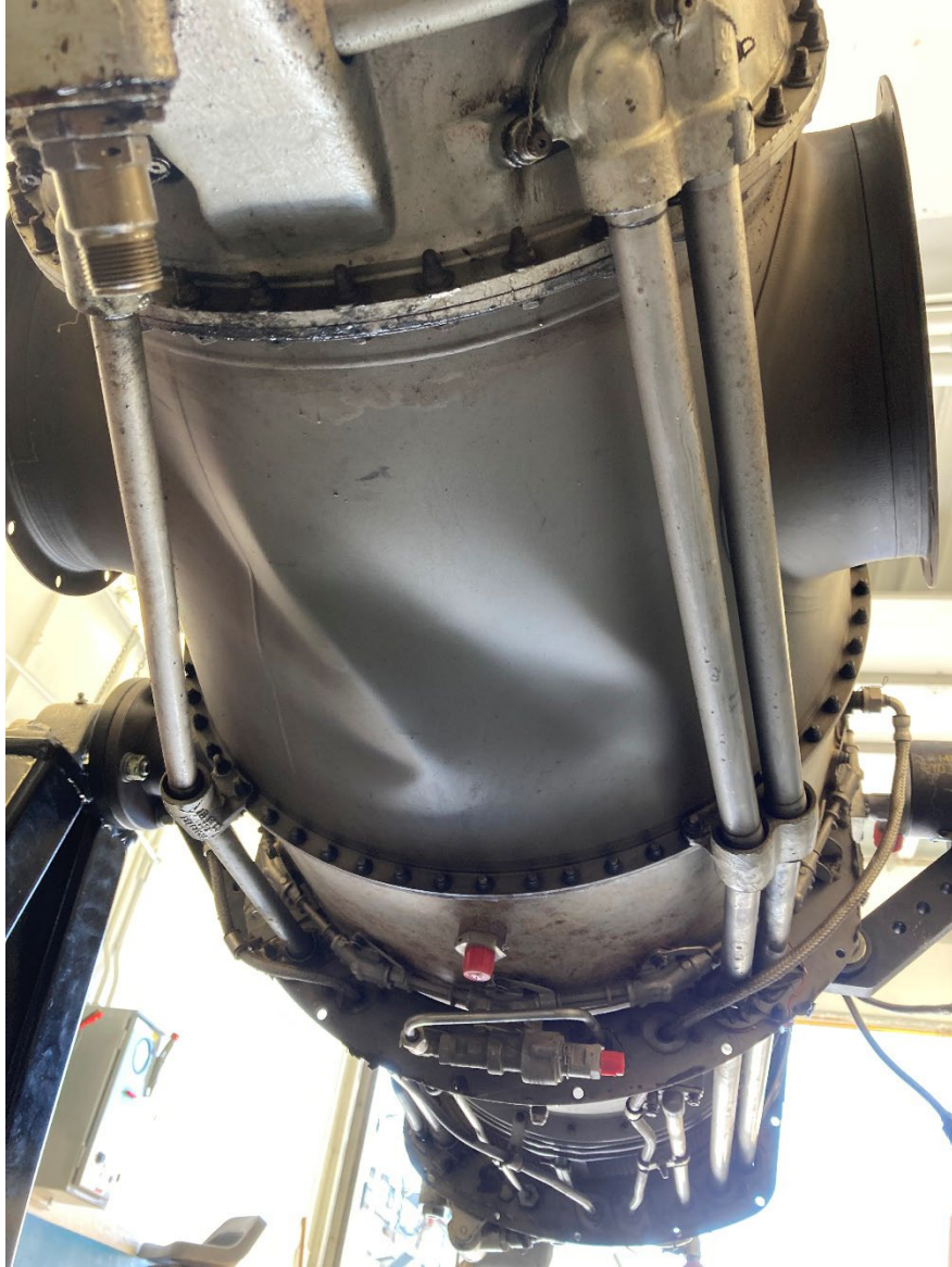
Figure 3. View of the bottom of engine with exhaust casing torsional buckling
