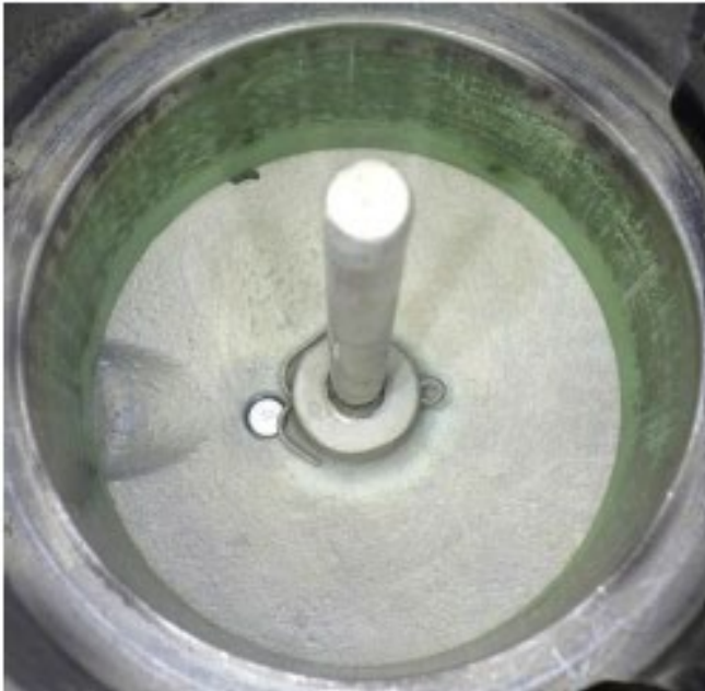
Photograph 6 - BOV piston removed from housing. (Courtesy of PWC)
