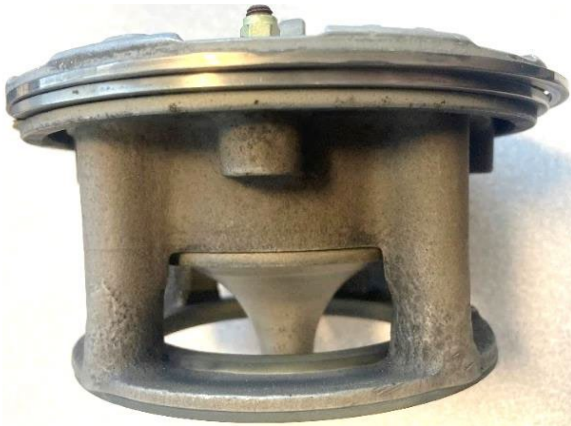
Photograph 4 - Compressor bleed-off valve removed. (Courtesy of PWC)
