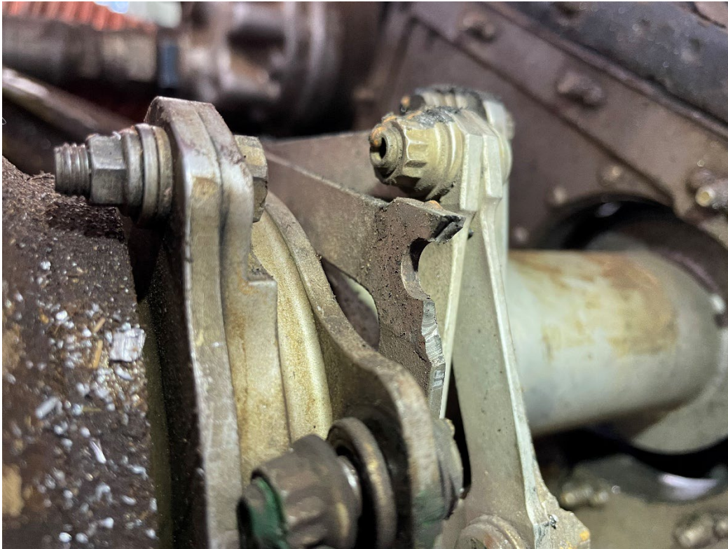
Figure 2. View of fractured KAflex plate.
