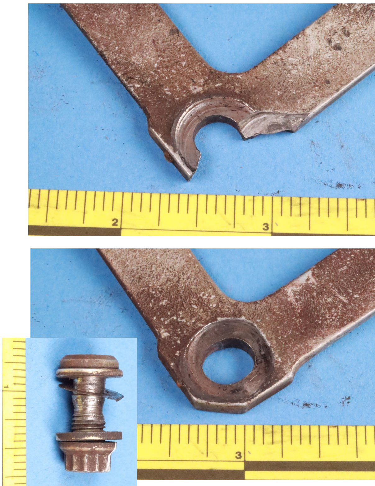
Figure 2. Aft face of the fractured flex plate after disassembly showing the fracture location (upper image) and the attachment hole on the opposite side of the plate (lower image). The hardware associated with the hole in the lower image is shown at the lower left side of the figure.
