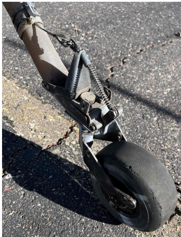
Figure 1 - Tailwheel assembly in locked position - note cable ties used to secure release cable.
