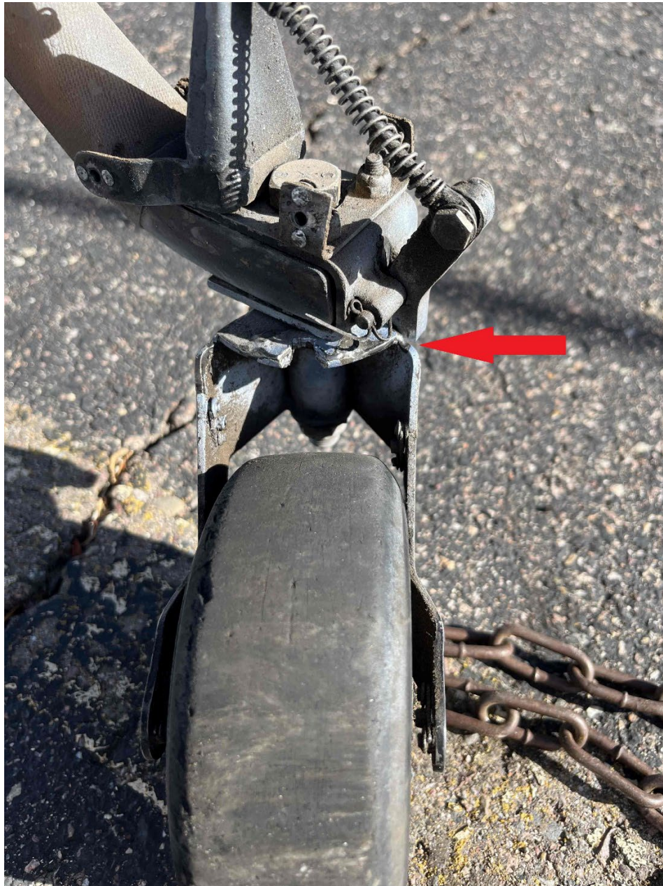
Figure 2 - Tailwheel about the 45 ° over center, with locking arm stuck past and against the pivot plate.
