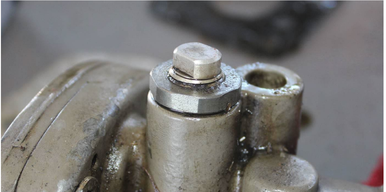
Figure 8: View of propeller governor mounting gasket stack with oil residue
