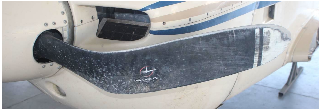
Figure 6: View of impact damage to propeller blade with about 45° aft bending, chordwise polishing and spanwise scratches
