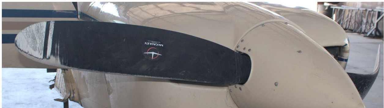
Figure 7: View of impact damage with slight aft bending to propeller blade chordwise polishing
