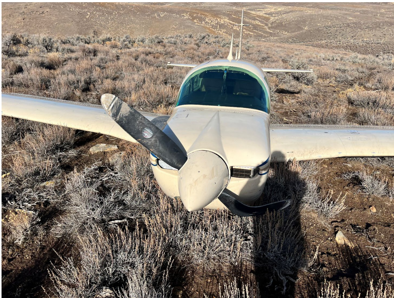
Photograph 1 - Forward to aft view of the accident airplane with propeller damage (Courtesy of FAA)
