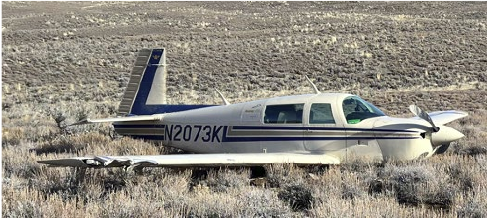
Photograph 3 - View of damage to outboard right wing and leading edge (Courtesy of FAA)
