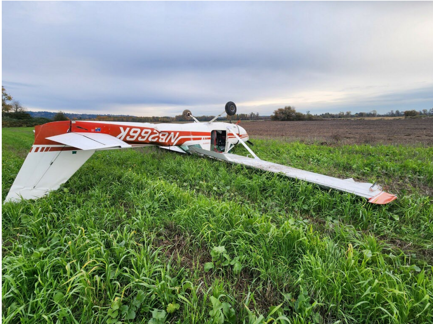
Photograph 1 - View of nosed over airplane with damage to aft fuselage (Courtesy of FAA)
