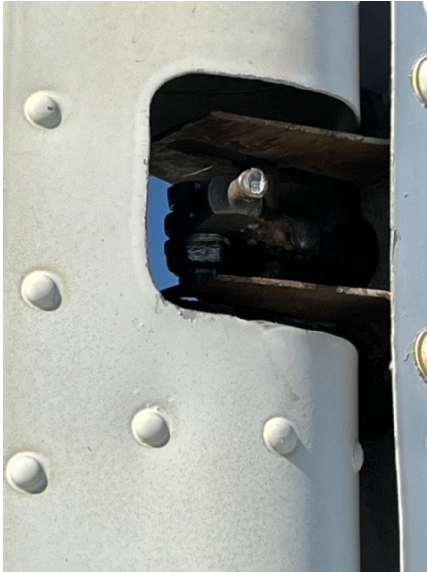
Photograph 3 - View of broken rudder trim tab rod end (Courtesy of FAA)
