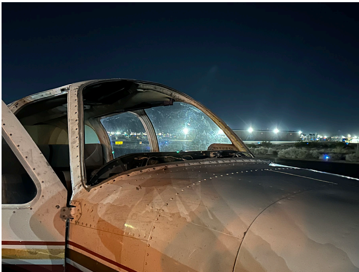
Photograph 1 - Front view of accident airplane with missing windshield (Courtesy of FAA)
