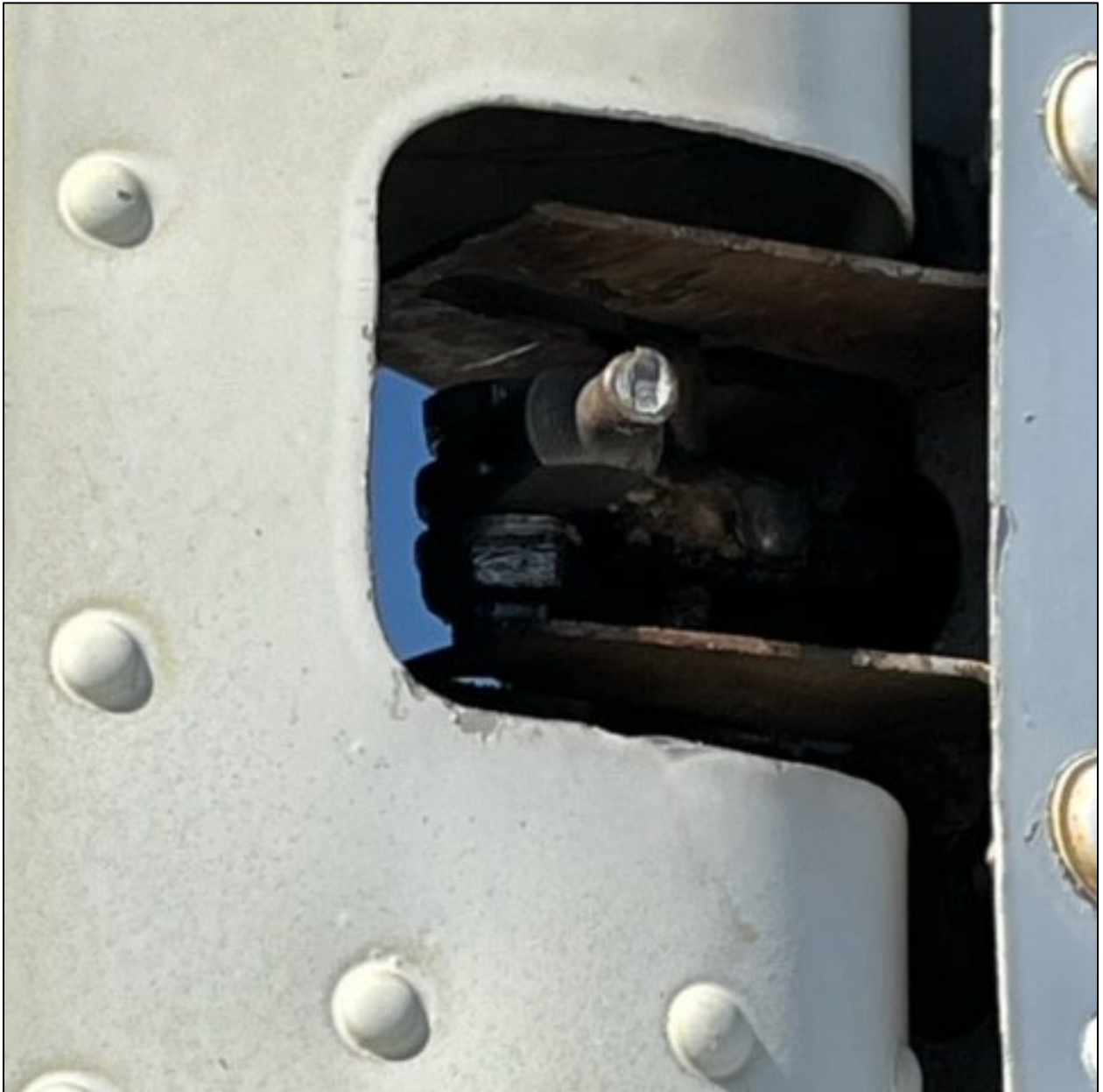
Figure 1: View of rudder trim tab rod end during examination
