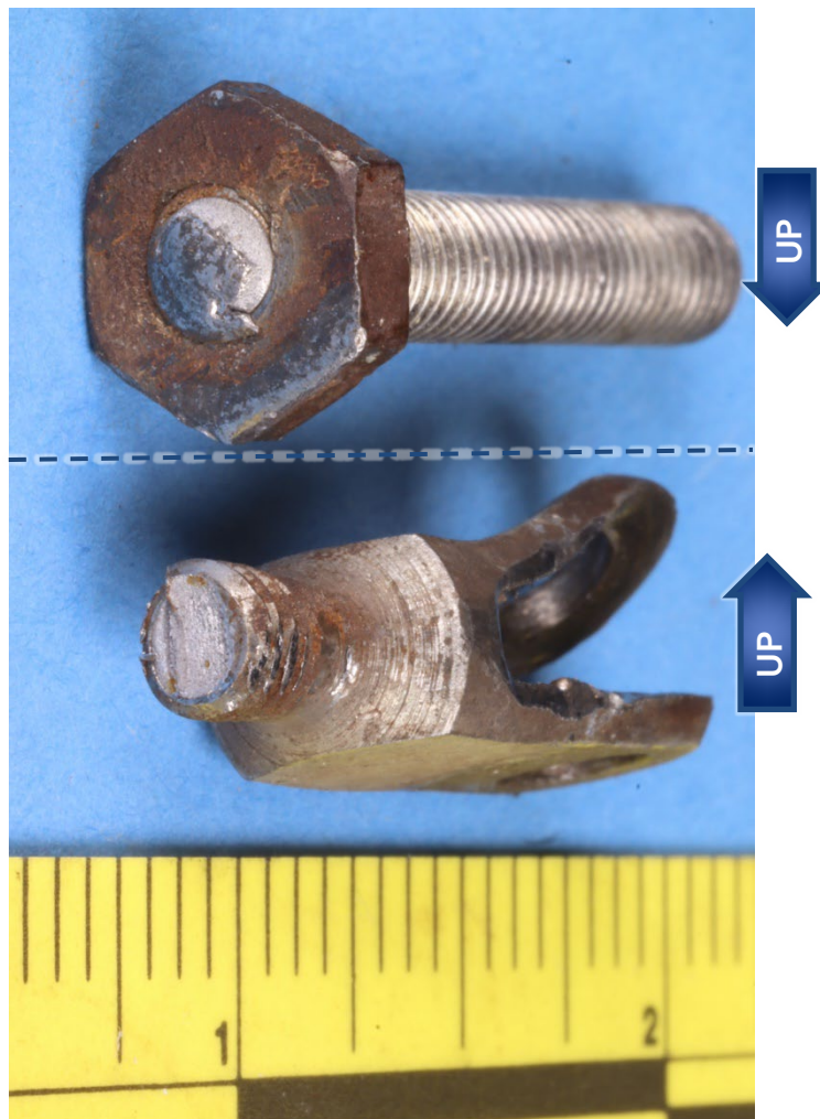
Figure 1. Overall views of the submitted rudder trim control rod end as received.
