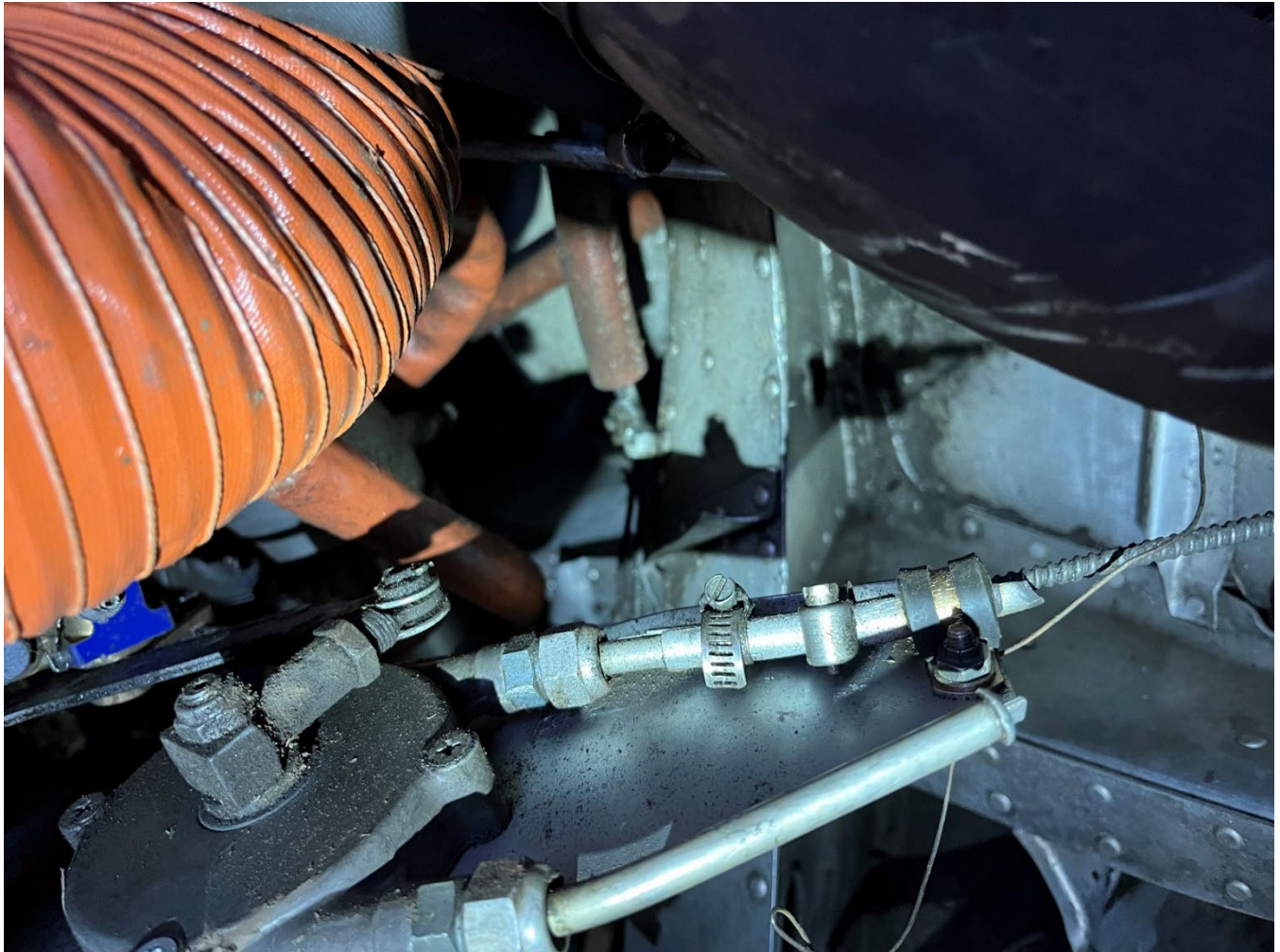
ASI-24-AD-022 (Fabricated cable clamp)
