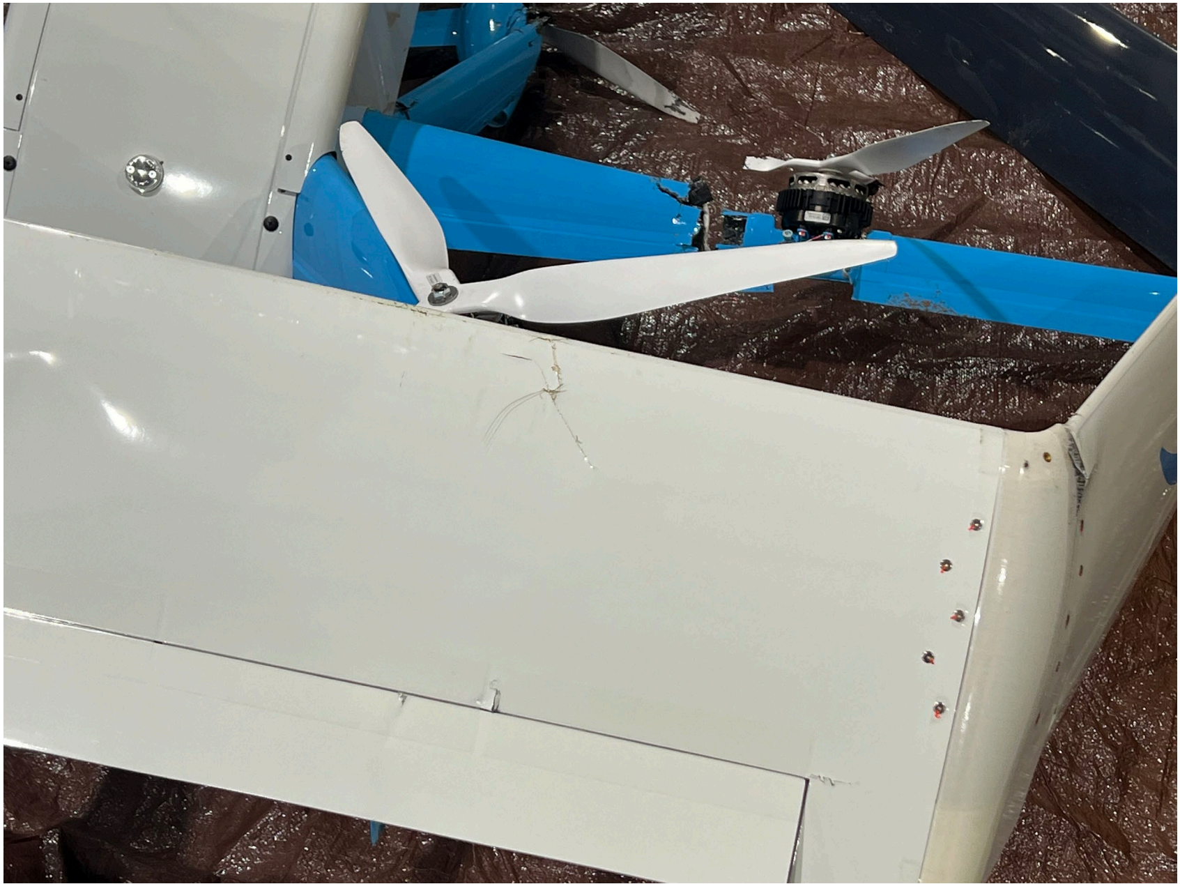
Photo 2 – View of upper wing damage (photo courtesy of operator)
