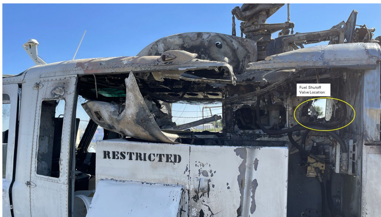
Photograph 3. Airframe Side Fuel Shutoff Valve
