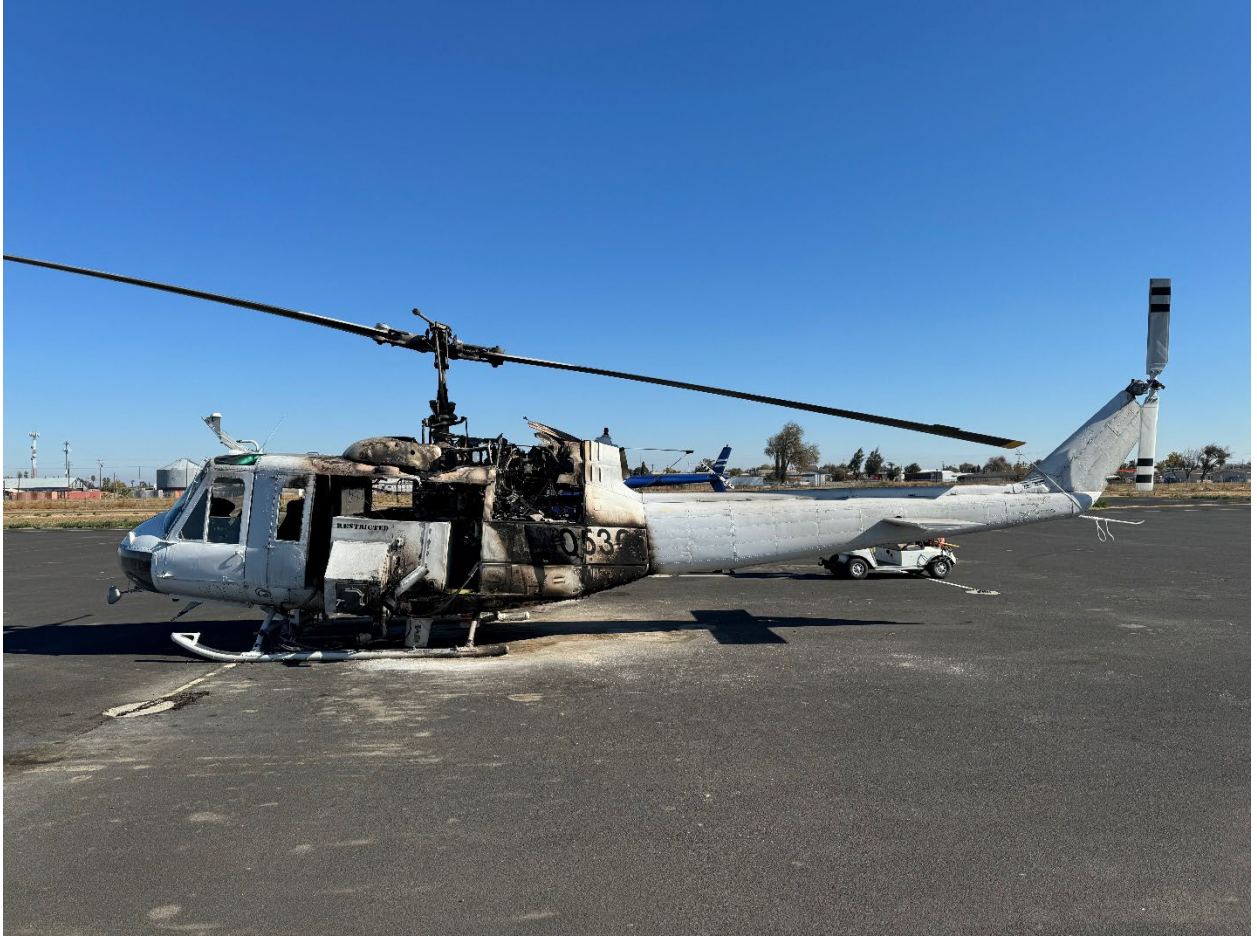
Photograph 1: Fire Damaged Left Side of Helicopter (Photo Courtesy of Insurance)
