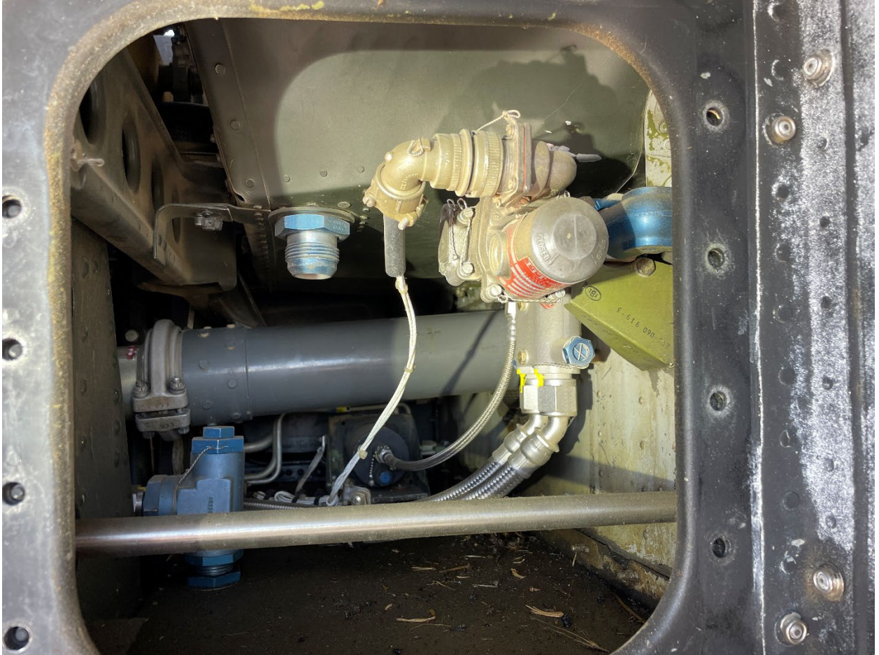
Photograph 4. Exemplar Fuel Shutoff Valve
