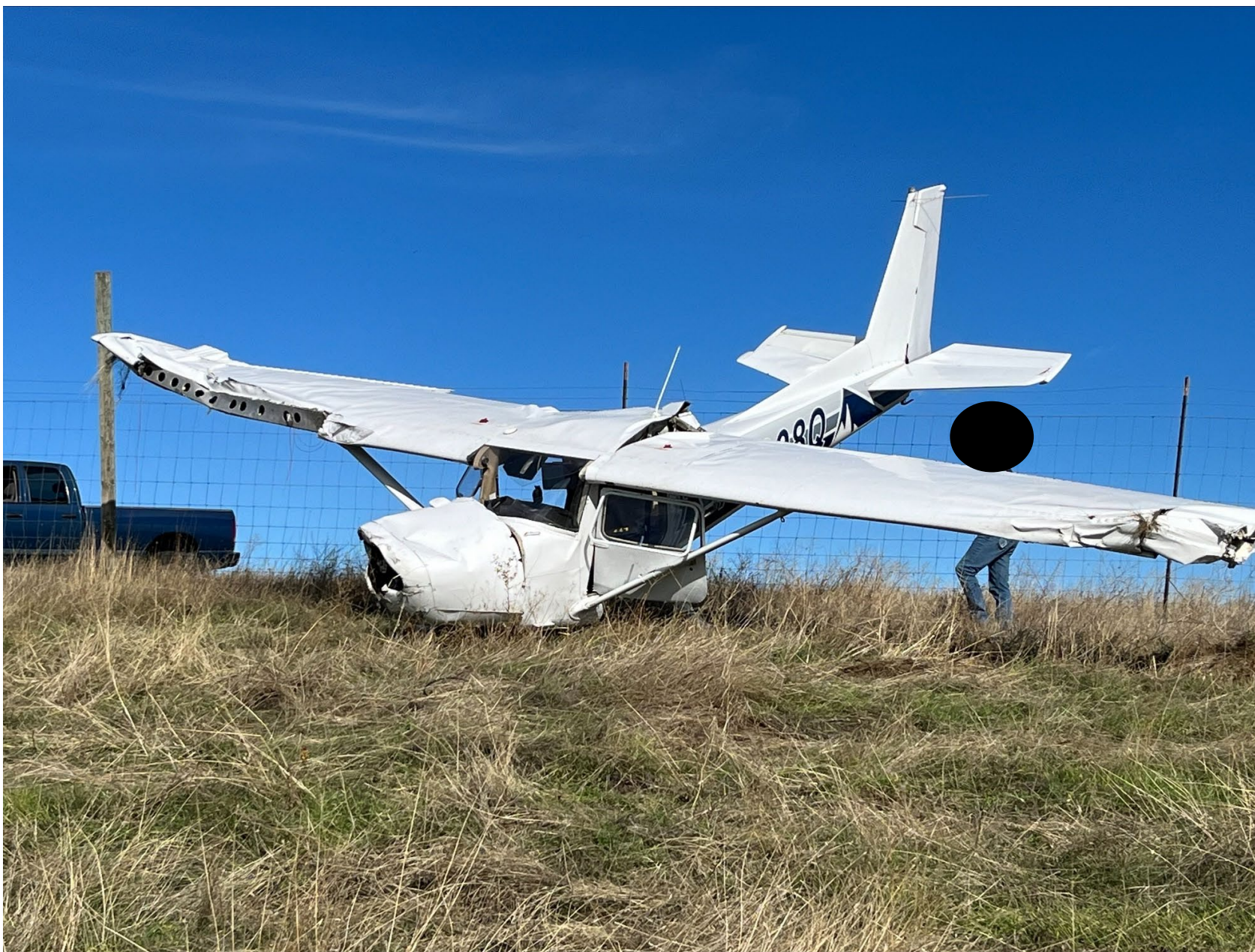
Photo 1 – View of damage to both wings and fuselage (courtesy of local law enforcement)
