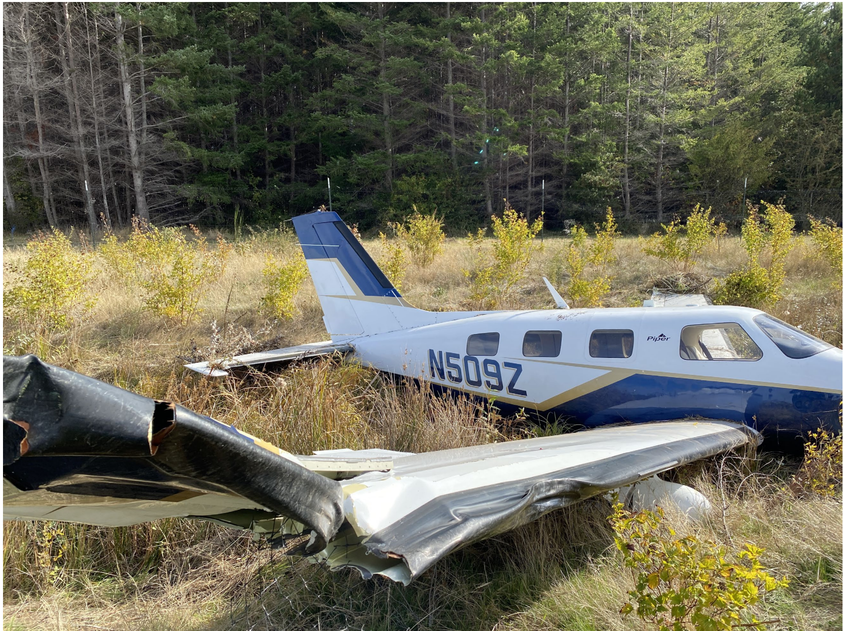
Photo 1 – View of right wing damage (Photo courtesy of San Juan Deputy)
