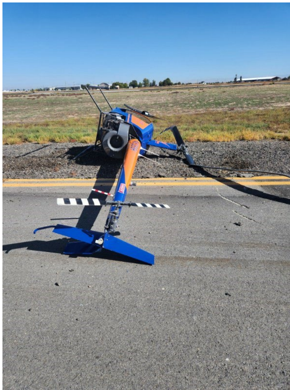
Photo 1 – View of damage to horizontal stabilizer (courtesy of Operator)
