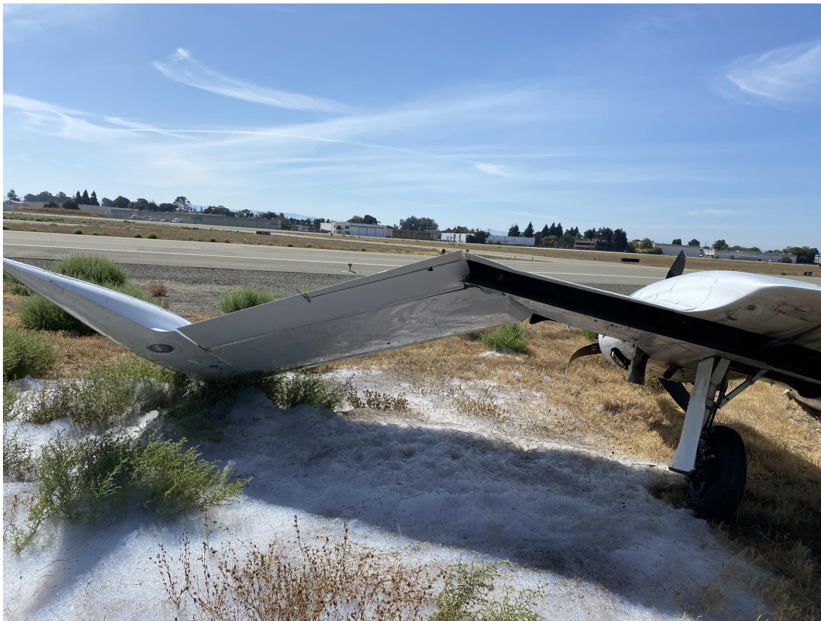
Photo 4 – Accident site, view of the left wing. (Courtesy of the Hayward Executive Airport)
