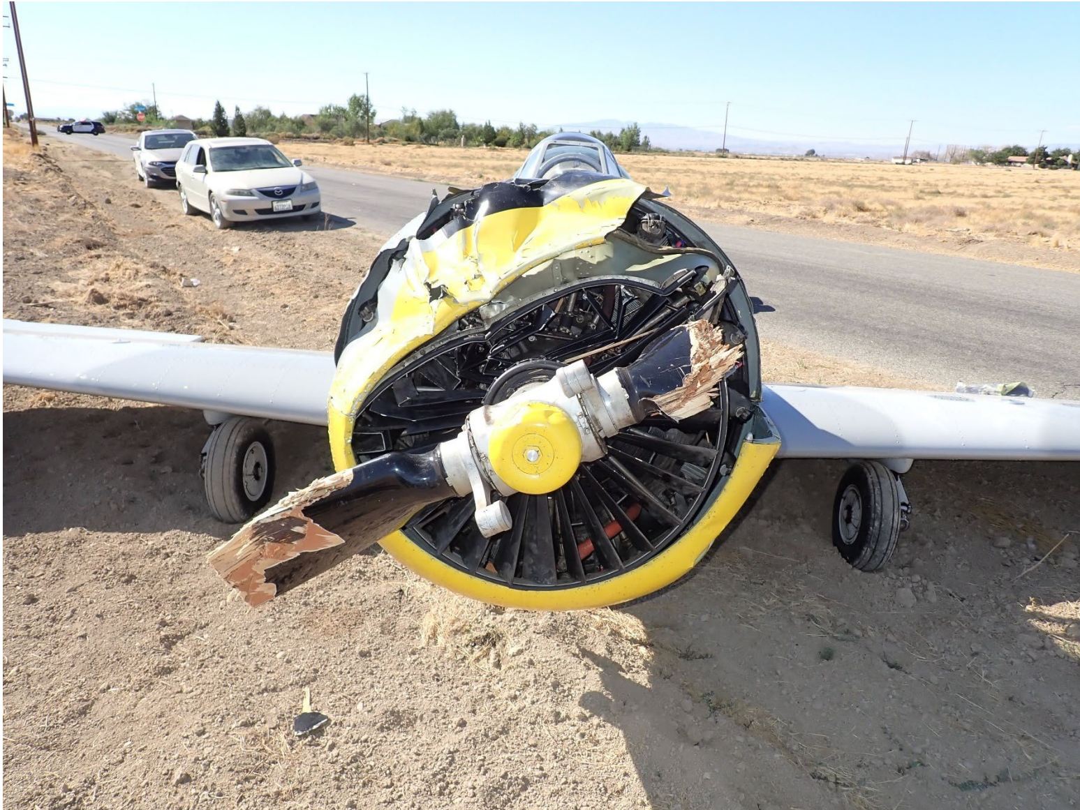
Photograph 8 - N5287 broken propeller blades at accident site
