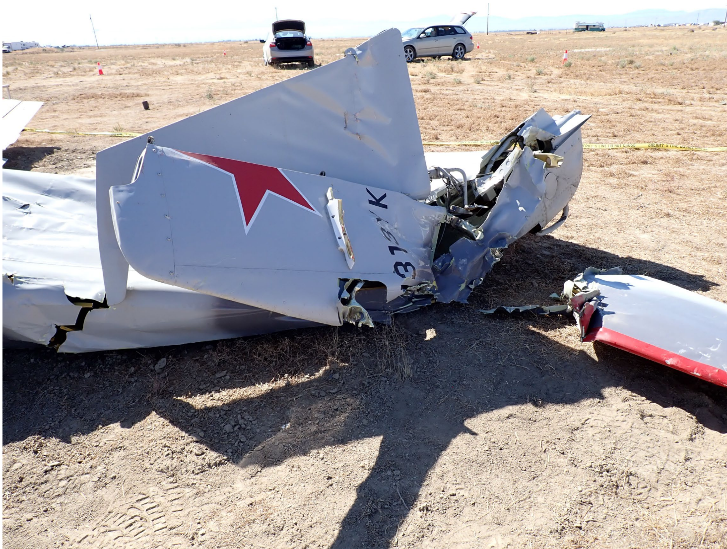
Photograph 4 - Partially separated vertical stabilizer from N313YK at accident site
