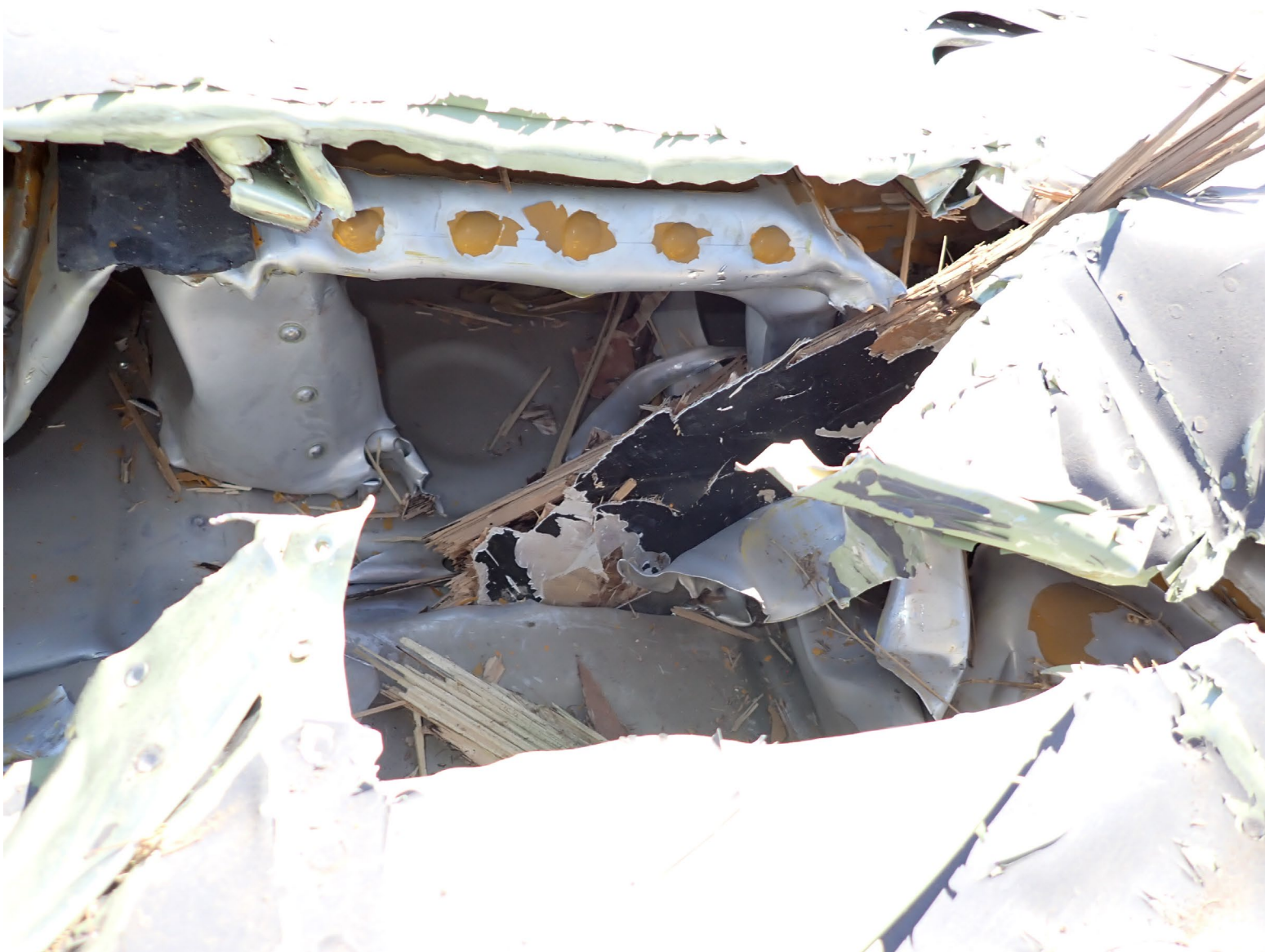
Photograph 3 - Propeller fragments in left wing of N313YK
