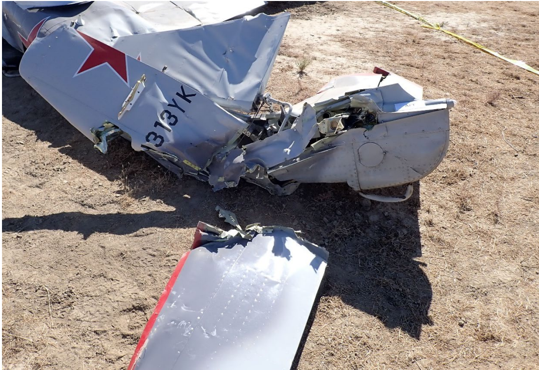
Figure 4: N313YK empennage from left side; note missing left elevator
