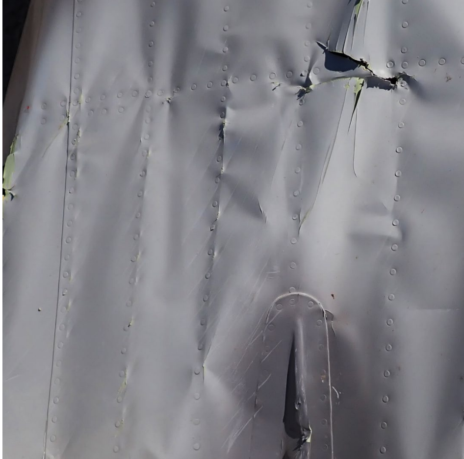
Figure 3: Light gray striated marks on top skin of aft fuselage (N313YK)
