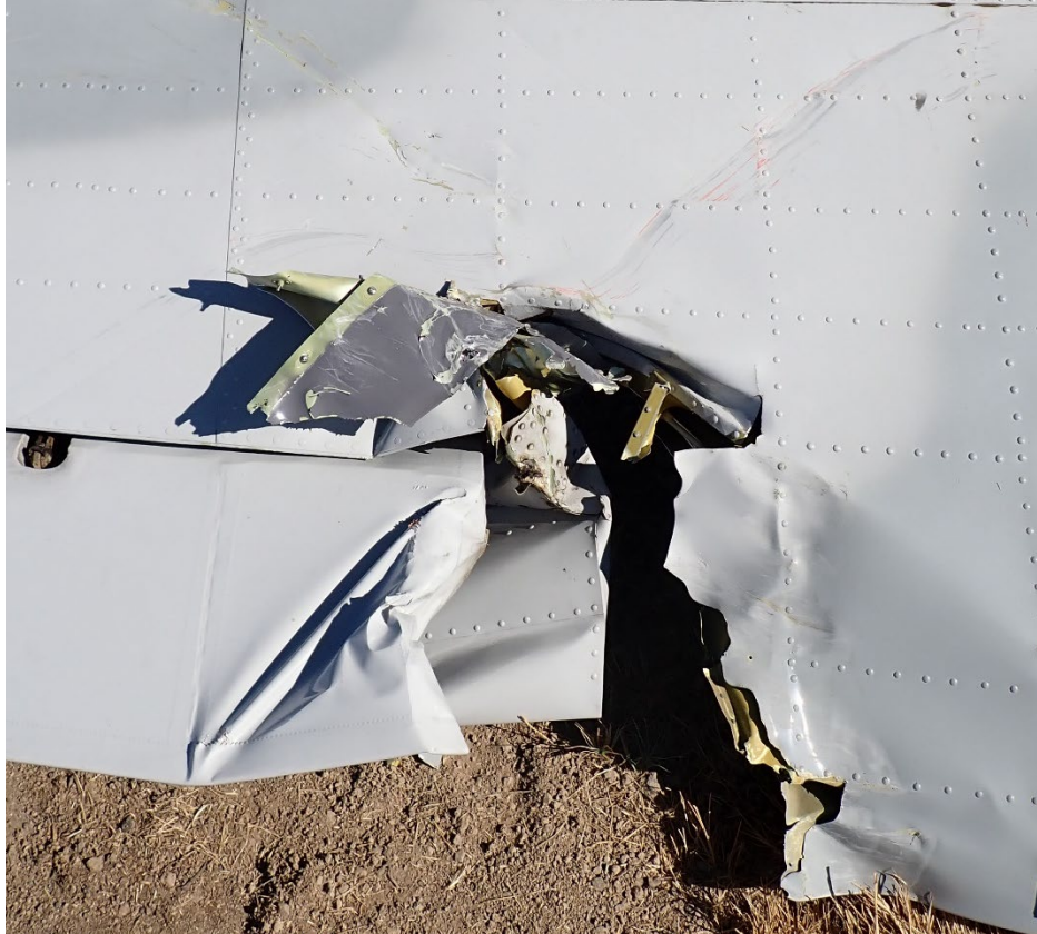
Figure 7: Damage to left wing trailing edge of N5287; note yellow and red paint transfer marks
