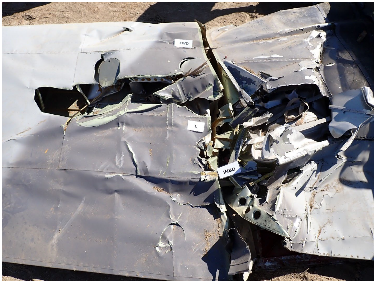
Figure 5: Damage to top skin of left wing on N313YK with embedded wooden propeller fragment
