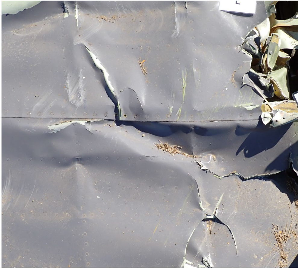
Figure 6: Yellow paint transfer marks on left wing (N313YK)
