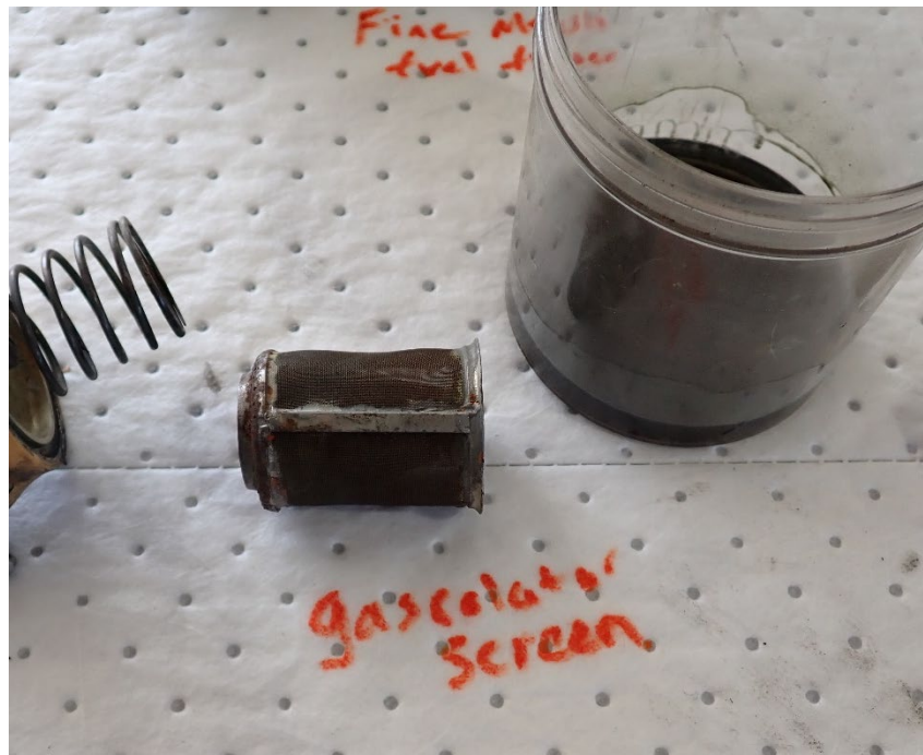
Figure 11: Gascolator screen and fuel sample from engine (N5287)
