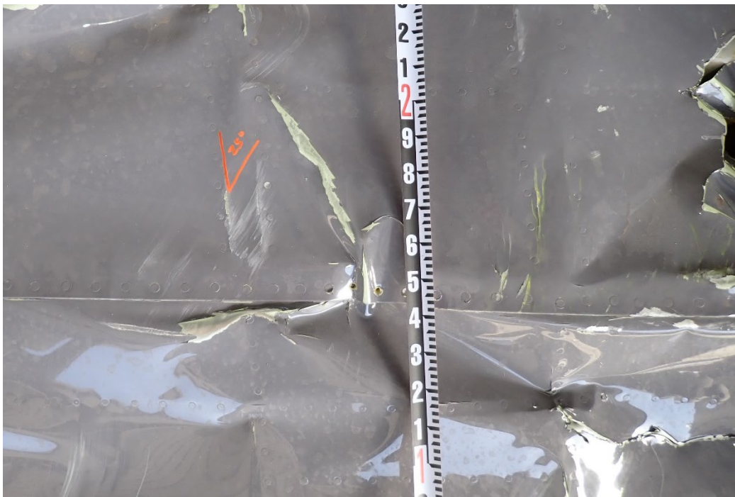
Figure 2: Yellow paint transfer marks and white/grey scuffing on left wing of N313YK
