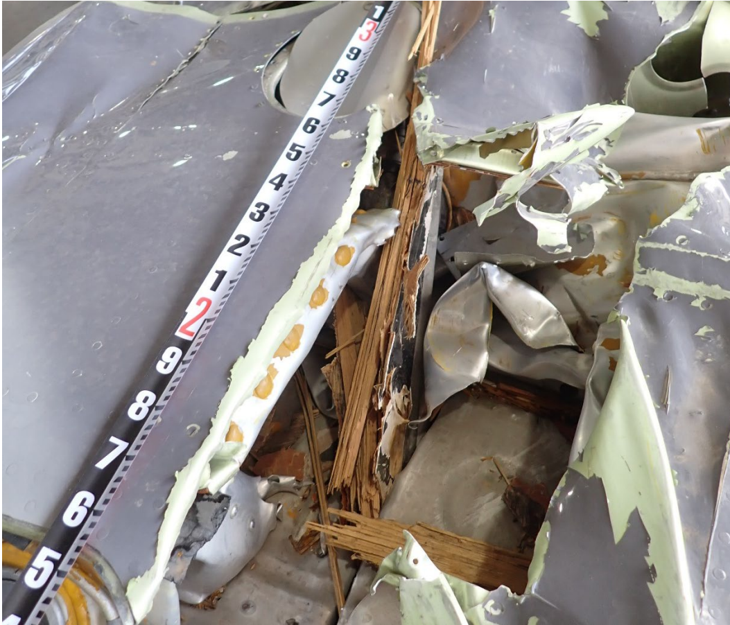
Figure 1: N313YK left wing with propeller fragments
