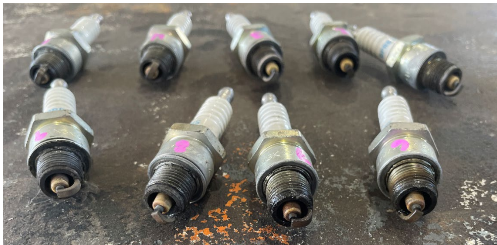
Figure 9: N5287 forward spark plugs
