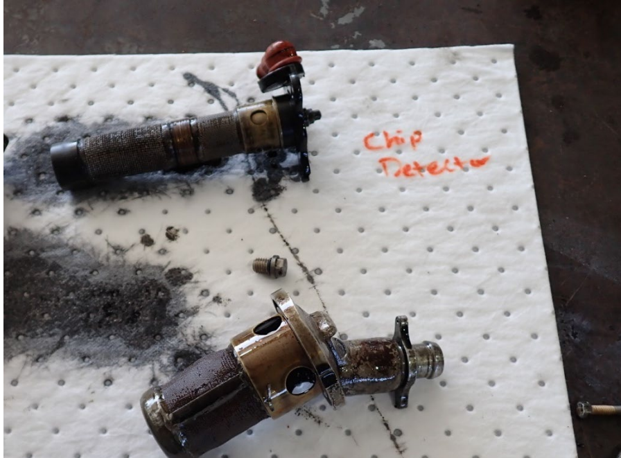
Figure 12: Oil inlet screen and chip detector from engine (N5287)
