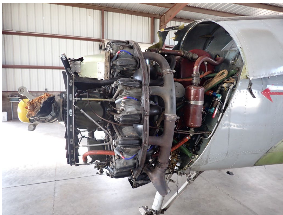
Figure 8: M-41P engine installed on Yak-52 prior to examination
