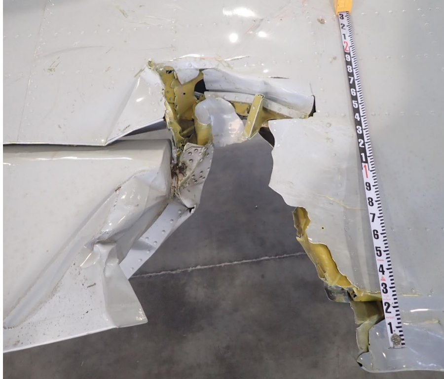
Figure 7: Left wing midspan trailing edge of N5287
