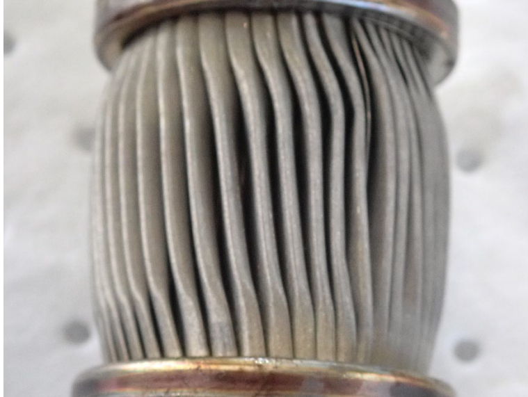
Figure 10: Metal fine mesh fuel screen from engine (N5287)
