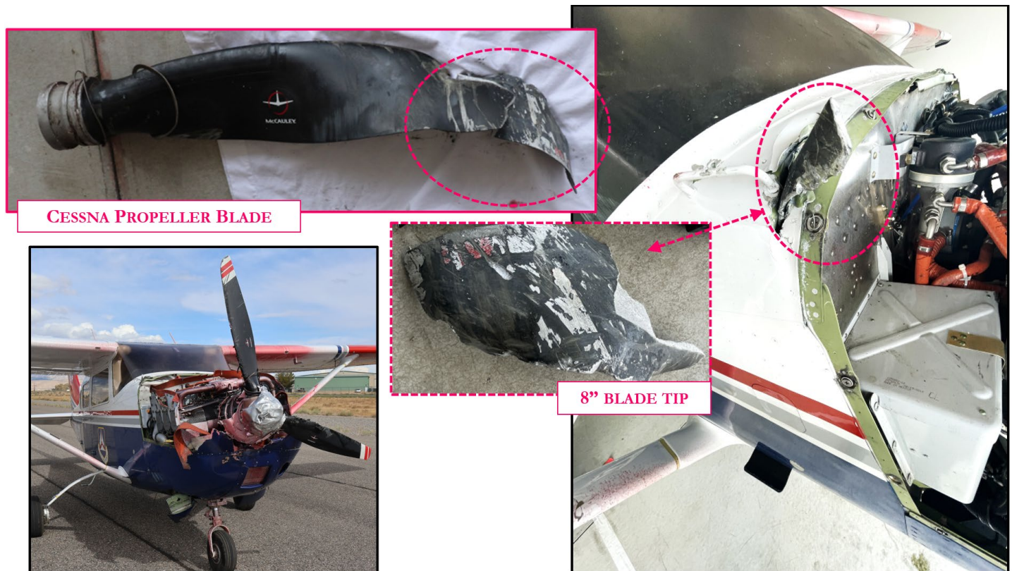
Figure 11: Impact damage showing Cessna propeller
