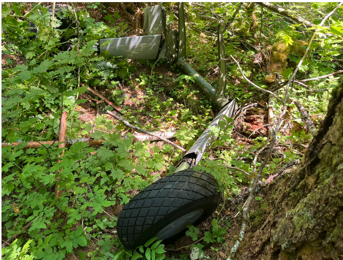
Photograph 5 - Main landing gear assembly. (Courtesy of FAA)
